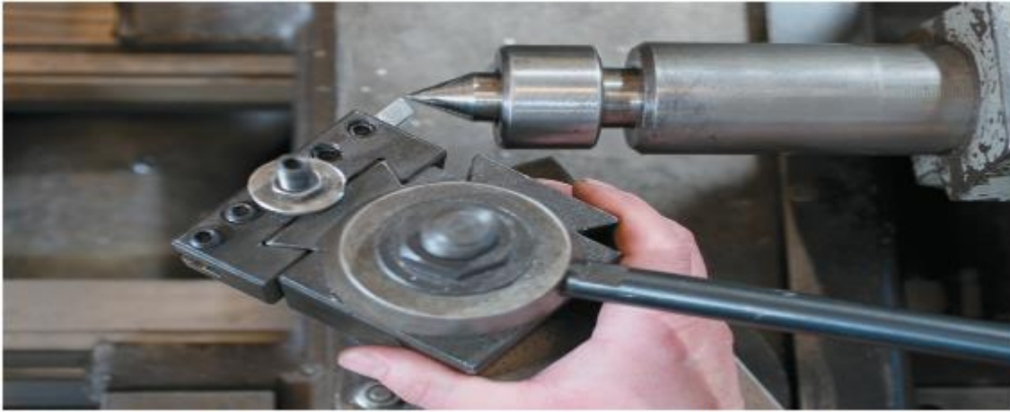
Setting the tool to the center of the workpiece using the tailstock center.
