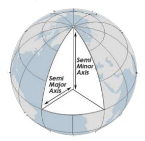
Reference ellipsoids are primarily used as a surface to specify point coordinates such as latitudes (north/south), longitudes (east/west) and elevations (height).
