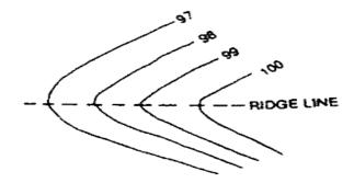
When the lower values are inside the loop, it indicates a valley line.Contour lines cross valley lines at right angles.
