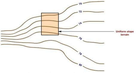
Contours of Terrain having different types of slope
