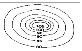
✓ Closely spaced contour indicates steep slope ground.
