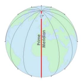
Together these lines provide a reference for latitude and longitude expressed in decimal degrees. These latitudes and longitude positions (Geographic Coordinate Systems) are based on a spheroid or ellipsoid surfaces that approximate the surface of the earth – a datum.
