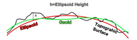
Ellipsoid height is the most basic version of up-and-down. The ellipsoid uses the size and shape of the **horizontal datum** such as WGS84. It gives a smooth surface without bumps or irregularities. The geoid is complex to describe it mathematically. Therefore, we fit different Ellipsoids to approximate it such as WGS84.
