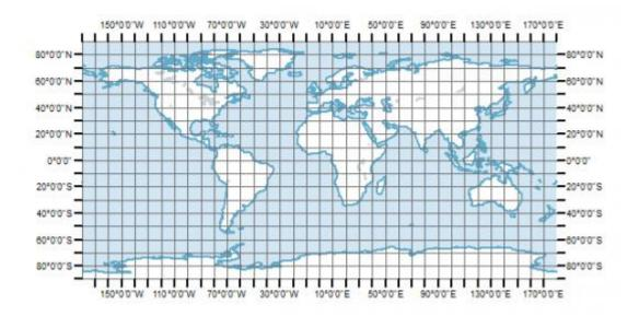
A datum describes the shape of the Earth in mathematical terms. A datum defines the radius, inverse flattening, semi-major axis and semi-minor axis for an ellipsoid.
