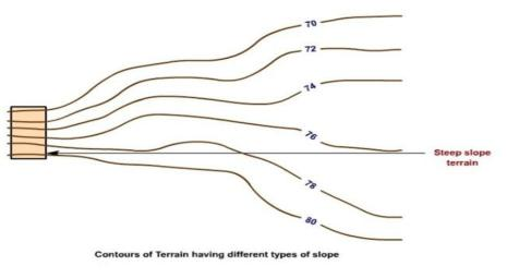
✓ Equally spaced contour indicates uniform slope.
