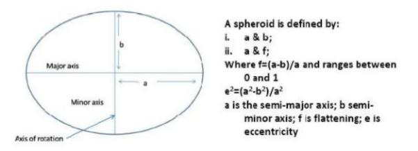
Different surveys of the earth have resulted in many spheroids representing the earth. Generally, a spheroid is chosen to fit one country or a particular area in order to have accurate mapping.
