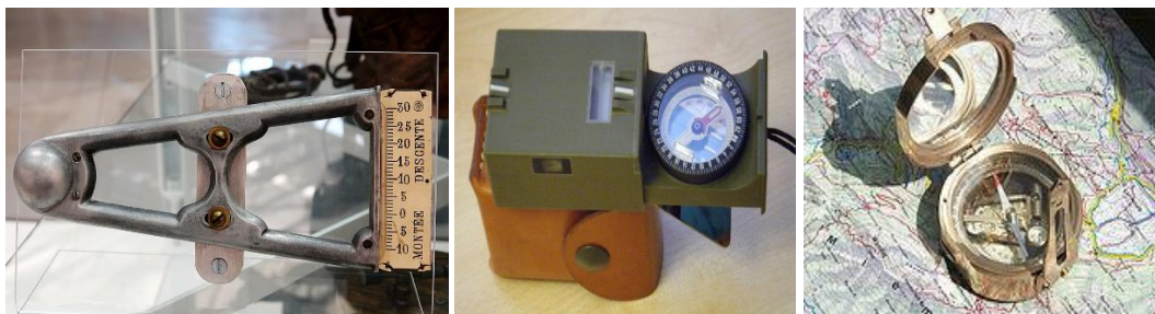
Figure 34: Mechanical tools (Blériot Monoplane Inclinometer, Military model and Compass with inclinometer)
