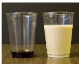
Figure 25 Undiluted and diluted emulsifiable concentrate formulation
