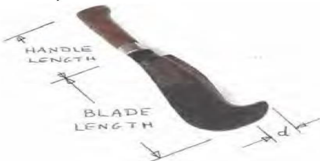
Principal dimensions to record for a billhook
