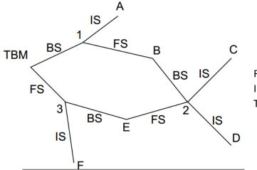
RL(TBM) = +50.000m Instrument stations: 1, 2, 3. Target points: TBM, A, B, C, D, E, F.
