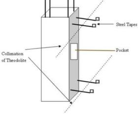
Checking Column Verticality Using Theodolite
