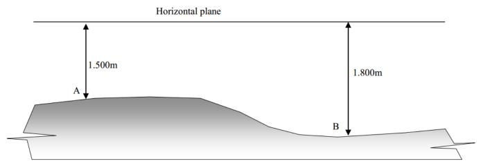
It can be seen in the above figure that point B is lower than point A and the difference in the measurement of 0.300m tells us the difference in level.
