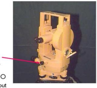
Optical Plummet Rotate to focus reticle  $\cap$ Pull in / out
