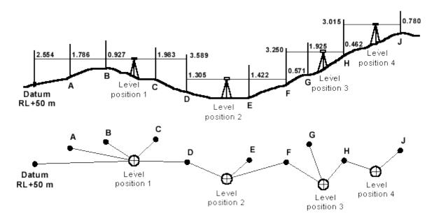
The leveling or field procedure that should be followed is shown in Figure below.
