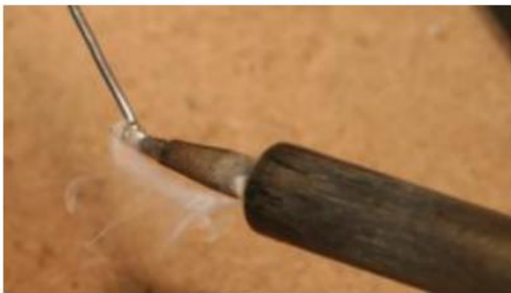
Apply Solder to Soldering Iron Tip
