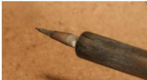
Properly Tinned Soldering Iron Tip
