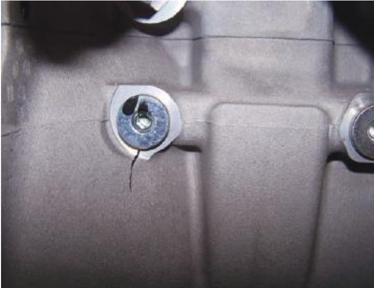
Figure 99 The topside oil artery crack appeared when an oxyacetylene flame was passed over the casting. Carbon in the flame was trapped in the crack, highlighting it.
