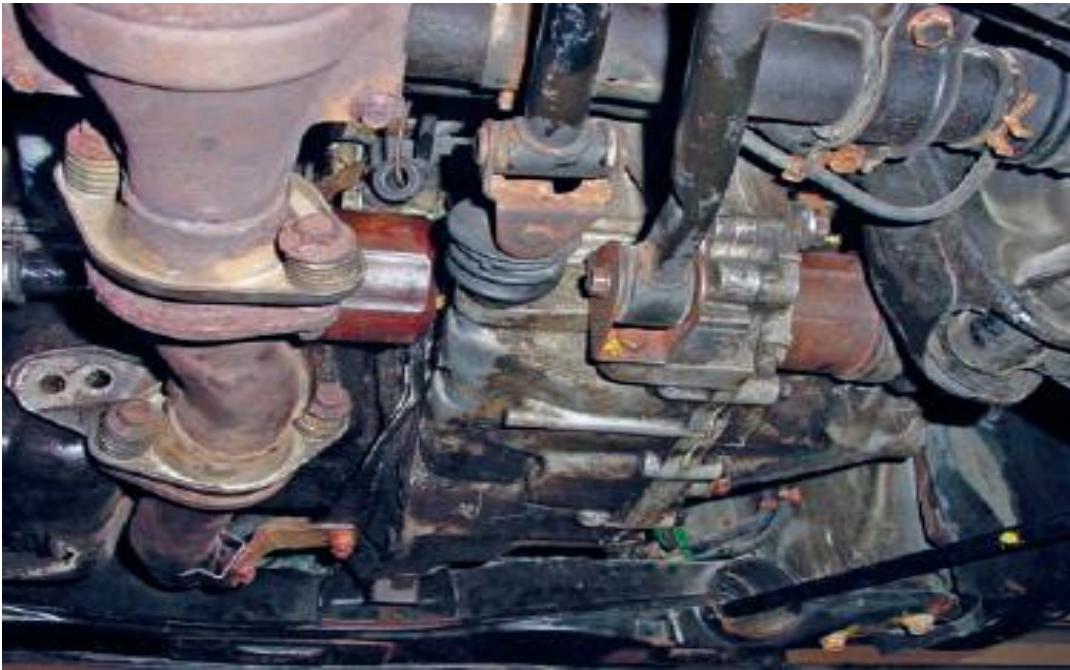
Figure 76 If the transmission will be removed with the engine, disconnect all linkages, lines, and electrical connectors.
