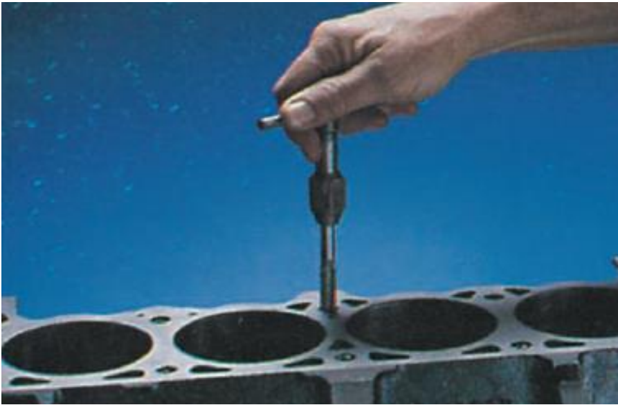
Figure 106 Cleaning bolt holes with tap. Used with permission of Detroit Gaskets
