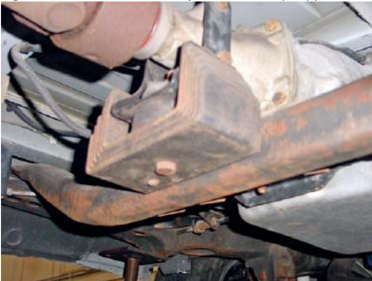
Figure 86 Use a transmission jack to securely support the transmission before removing the motor mounts.
