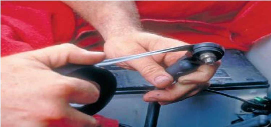
Figure 75: After the negative battery cable is disconnected, tape the terminal end to prevent it from accidentally touching the battery.
