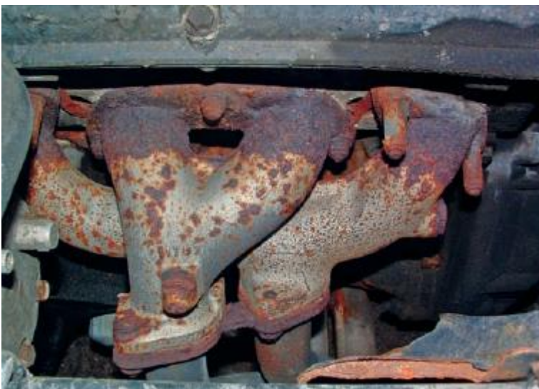
Figure 81 The exhaust system must be disconnected to remove the engine. Often this is the condition
