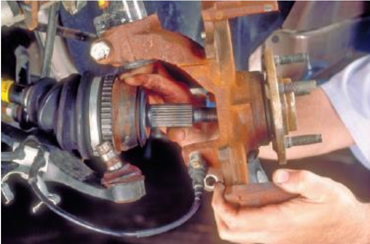
Figure 84 Pull the steering knuckle outward to allow the CV joint shaft to slide out of the hub.
