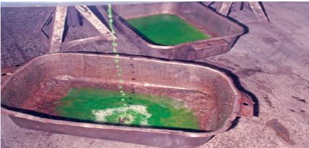
Figure 77 Drain the engine's coolant and recycle it.
