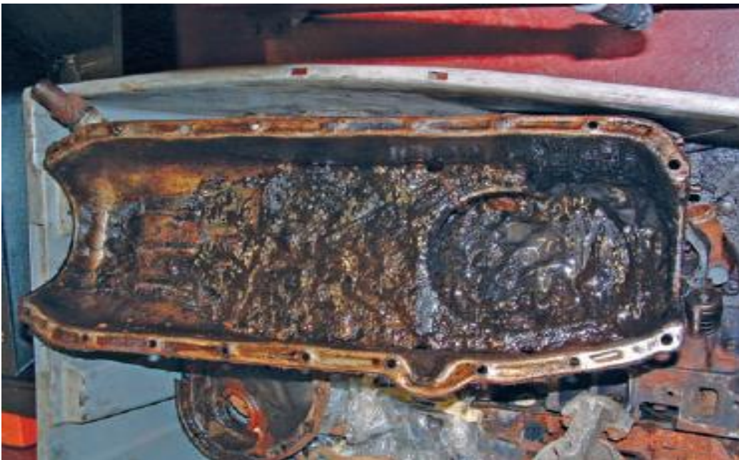
Figure 96 A major buildup of sludge on the bottom of this oil pan.
