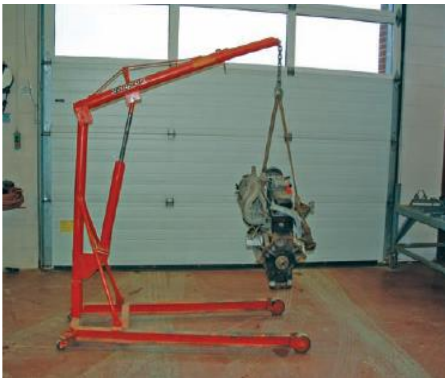
Figure 88 Once the engine is removed and is hanging on the engine hoist, lower it close to the floor so it can be safely moved to the work area.
