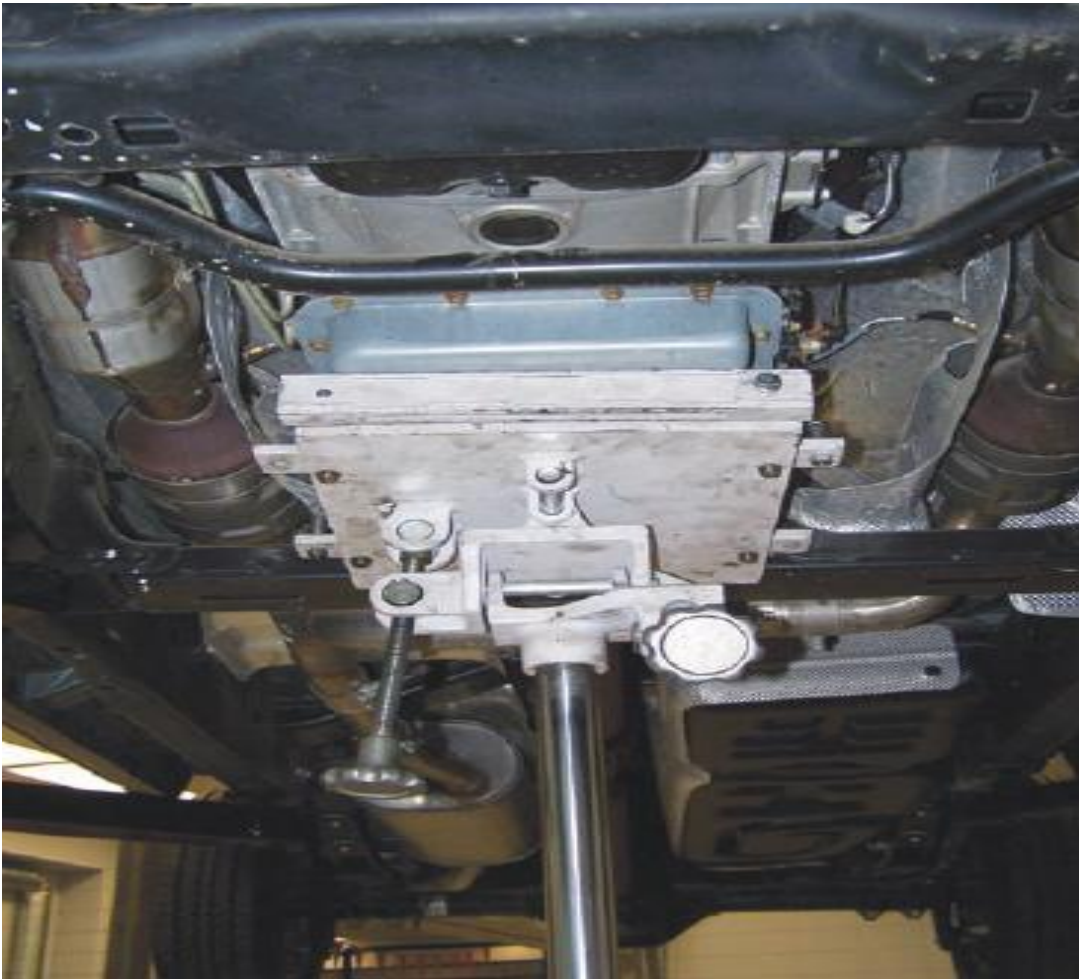
Figure 86 Use a transmission jack to securely support the transmission before removing the motor mounts.
