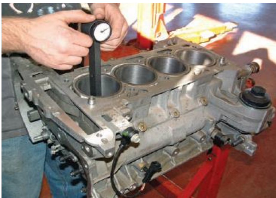
Figure 103 Cylinder bore is checked for outof- oundness with a dial bore gauge.
