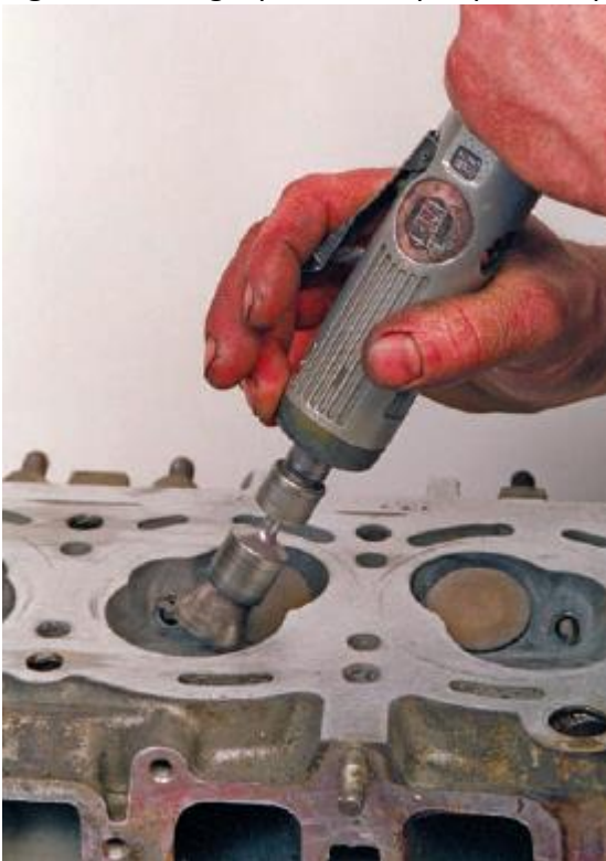
Figure 90 Carbon can be removed with a wire wheel driven by an electric or air drill motor.
