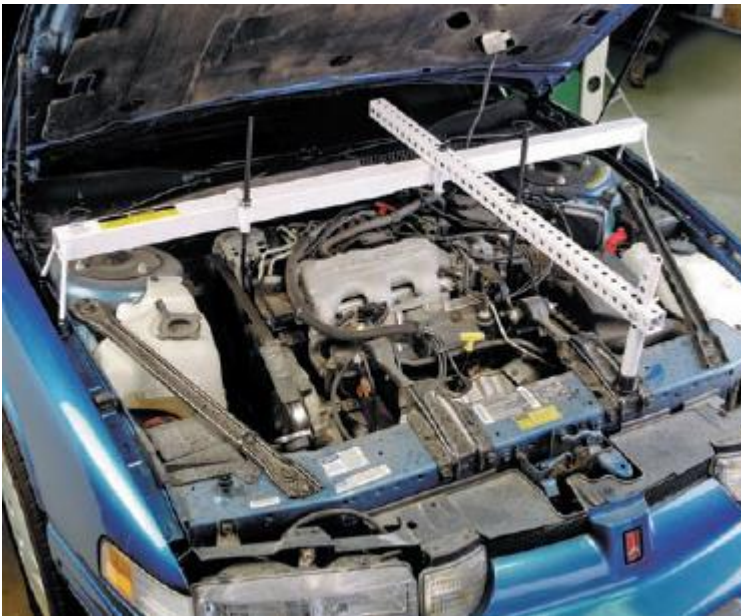
Figure 82 A transverse engine support bar provides the necessary support when removing an engine from a FWD vehicle. Courtesy of SPX Service Solutions
