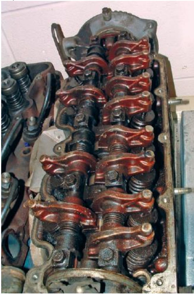
Figure 93 Remove the valve cover and disassemble the rocker arm components. Check the rocker area for sludge. Keep the rocker arms or rocker arm assemblies in the order they were installed.
