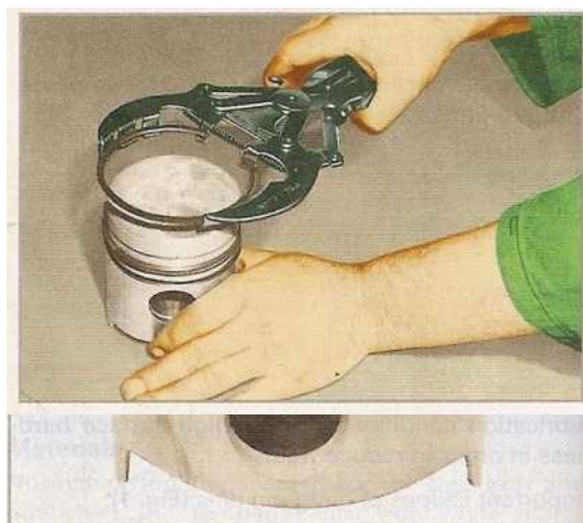
Figure38: installation of piston ring
