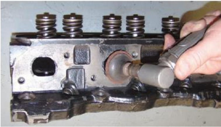
Figure 89 Using a power scraper pad will prevent any metal from being removed.
