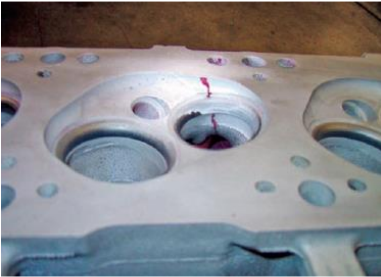
Figure 100 Cracks appear as red lines when a dye penetrant is used. Courtesy of LOCK-N-STITCH Inc.
