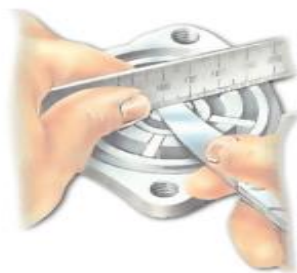
Figure 44 measuring gap between vanes and rotor
