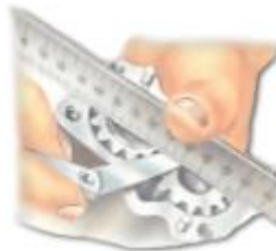
Figure 41 Check the gap between the straight-edge and the face of the two gears.
