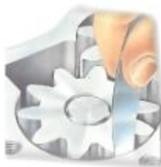
Figure 42 rotate the gears, and measure the gap between each tooth and pump body.
