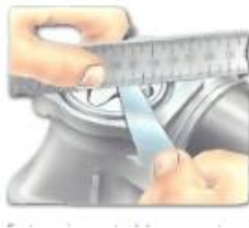
Figure 39 checking the clearance
