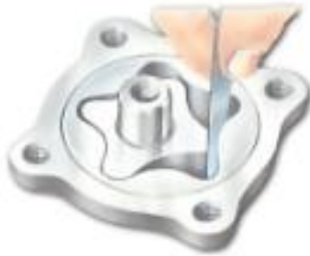
Figure 40 checking the clearance between the tips of the inner and outer rotor lobes.
