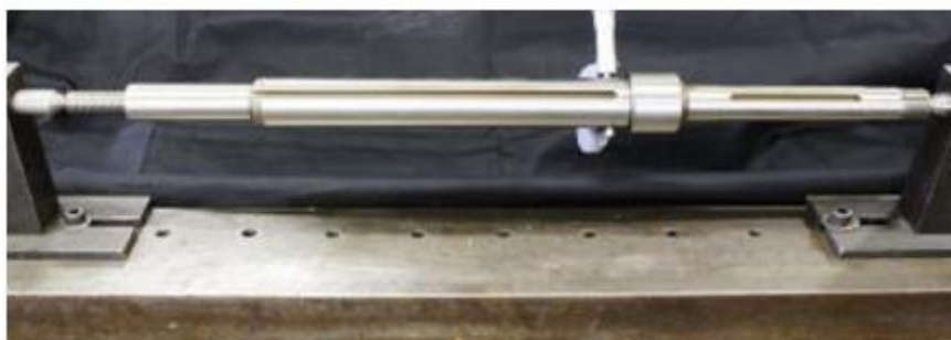
Figure 145.step measure the shaft closet to the tooling shoulder
