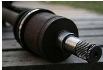
Figure 10. Splines on a front drive axle.
