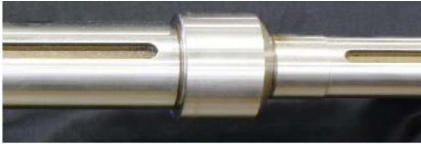
Visually inspect keyways for chips
