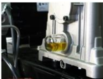
Figure 151.Oil level, color and clarity at all sight glasses
