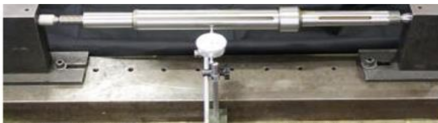
Step 4: Use dial indicator at the center portion of the shaft to check for runout
