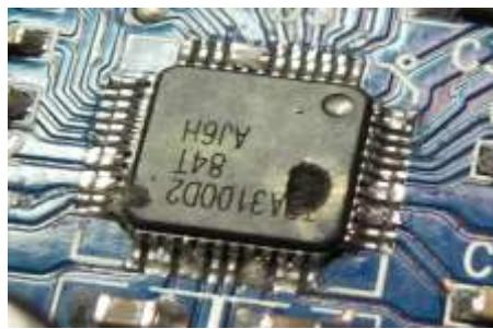
In this method you have to test an ic that weather the package is damaged. Take the observation of the ic from each of the sides possible, if you see even a little crack, burned mark or its broken from either side then the ic is surely to be damaged or leaked.
