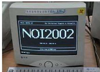
The first computer monitors and the TV receiver screen used cathode ray tubes (CRTs). One electron beam was used to produce the picture, the electron beam is made of white phosphorus which only allows it to produce black and white images. The display was monochrome and far less sharp and detailed than on a modern flat-panel monitor. CRT monitors have a superior response time.
