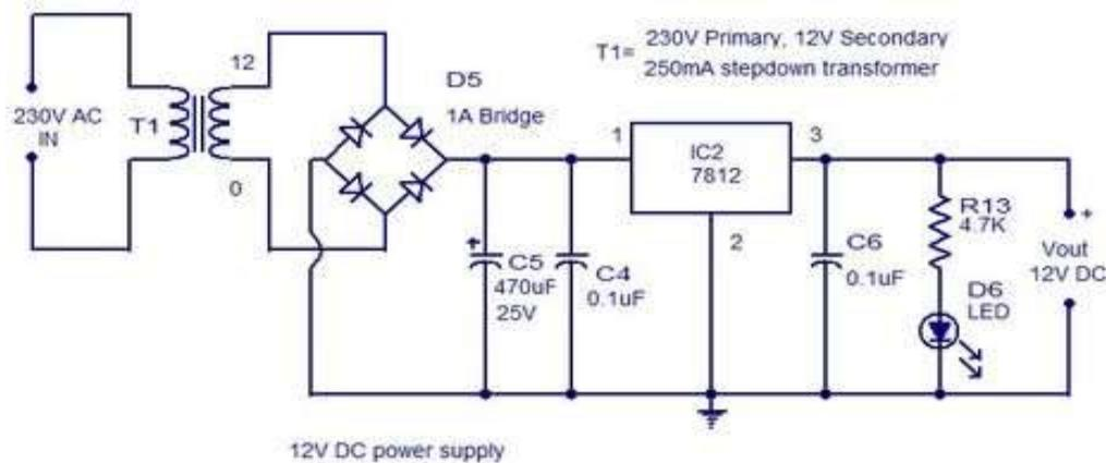
i. **Transformer**, a transformer is a static piece of equipment used either for raising (step up) or lowering the voltage of an AC (step down). It essentially consists of two windings, the primary and secondary. The winding connected to the AC Source is called primary winding (or primary) and the one connected to load is called secondary winding (or secondary).
