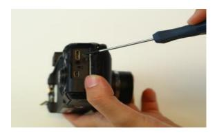
Remove the screw on the right side of the view finder on the back side of the camera.
