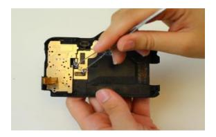
Using precision tweezers, pry the old function dial out of its socket leaving only a black, metal ring attached.
