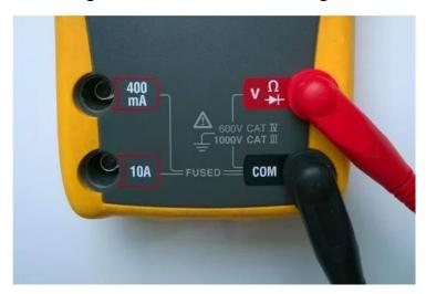
Test leads and 4mm sockets on a DMM, setup to measure voltage
