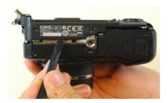
The back case is still attached to the camera with a yellow ribbon cable. The socket has a black flip-up lid that must be flipped up before the cable can be removed. Use precision tweezers to remove the cable.
