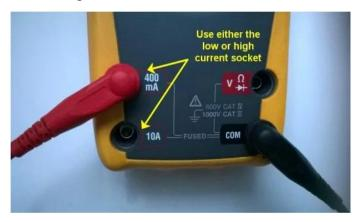
Test leads and sockets on a DMM, setup to measure current | Source
