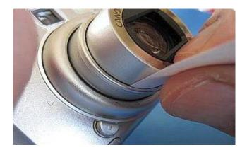
If your camera gives you a lens error message, the first thing to try is to clean out the lens area. Use a can of compressed air (sold at electronics stores for this purpose) to clean out all the pieces, paying particular attention to where the lens retracts and any area where it would be easy for dirt to get stuck in. You can also use a hair dryer set to the no heat setting.
