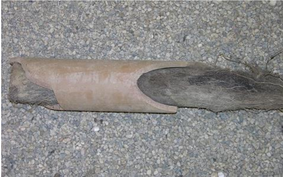
Figure: Drain pipe plugged with tree roots
