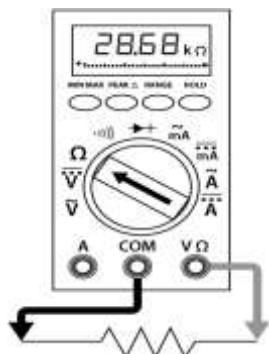
✓ **Resistance measurement using Color coding**
