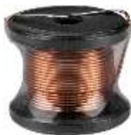
The coil is wrapped around the cylinder. The bobbin core does not provide a closed magnetic path; instead, the flux goes through the disc into the air gap and then enters the core through the second disc at the other end. It provides a large air gap for its magnetic field to store more energy, which increases the inductor's saturation current.
