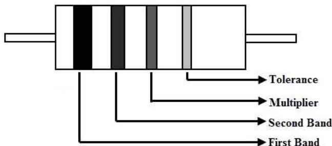
The above figure shows the 4-band inductor consisting four different color bands. Similar to the number coding, first and second color bands represents the first and second digits of the value, third color band is the multiplier and fourth band is the tolerance.
