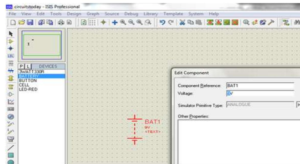
**Step6. Simulate the Circuit:** After completing the design, go to **Debug > Run Simulation** or click the play button in the toolbar.
