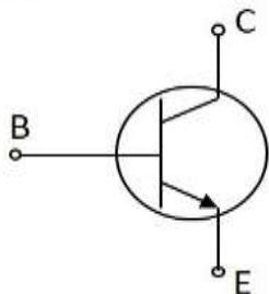
The types of BJT are NPN and PNP transistors. The NPN transistor is made by placing a p-type material between two n-type materials. The PNP transistor is made by placing an n-type material between two p-type materials.
