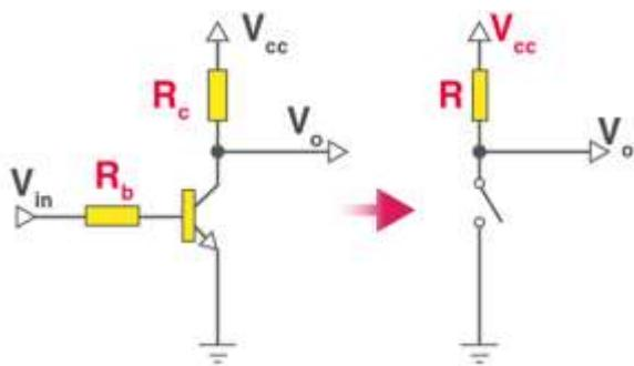
Some devices, including LEDs, only require several milliamperes of DC voltages at the logical level and can be directly controlled via the logical gate output. High-power devices such as generators, solenoids or lamps usually need more power to use transistor switches than the usual logic gate.
