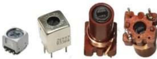
The most common design of variable inductors is having a movable ferrite core. Moving the core along the winding will increase or decrease the permeability which affects the inductance. The core can be designed to slide or screw in or out of the coil.
