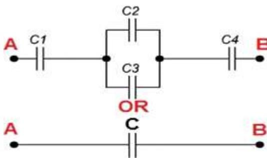
When calculating the total capacity of such a circuit section with a series-parallel connection of capacitors, this section is divided into the simplest sections consisting only of groups with series or parallel connections of capacitors. Further, the calculation algorithm is as follows:
