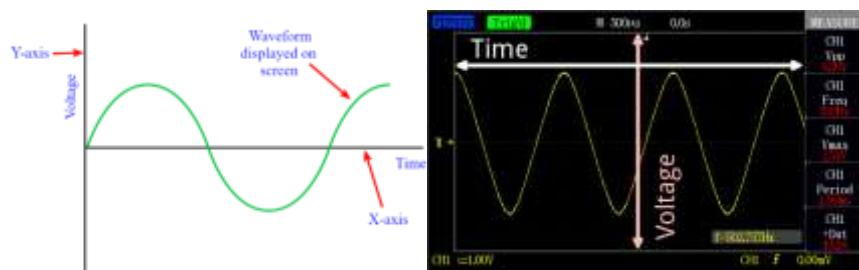
The oscilloscope is one of the most important electronic instruments available for making circuit measurements. It displays a curve plot of time-varying voltage on the oscilloscope screen.
