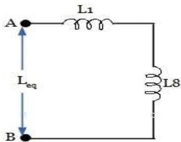
In the reduced circuit, the inductors L1 and L8 are in series.
