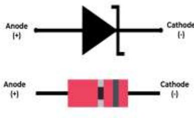
Zener diode can provide a stable reference voltage. These diodes can be operated in reverse biased and break down at a certain voltage. These diodes are mostly used in power supplies to provide a reference voltage.
