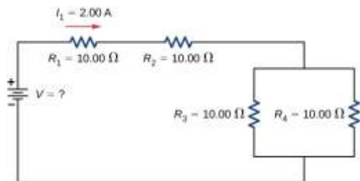
b) To reduce the circuit, first consider the two resistors in parallel.
