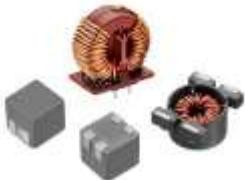
**Uses:** They have multiple applications depending on their winding. 1:1 winding ratio inductors are mostly used for electrical isolation or increasing the series inductance. The winding ratio of 1: N coupled inductors (which can step up or step down voltages) are used in other energy conversion circuits such as fly back, SEPIC, ZETA, etc.
