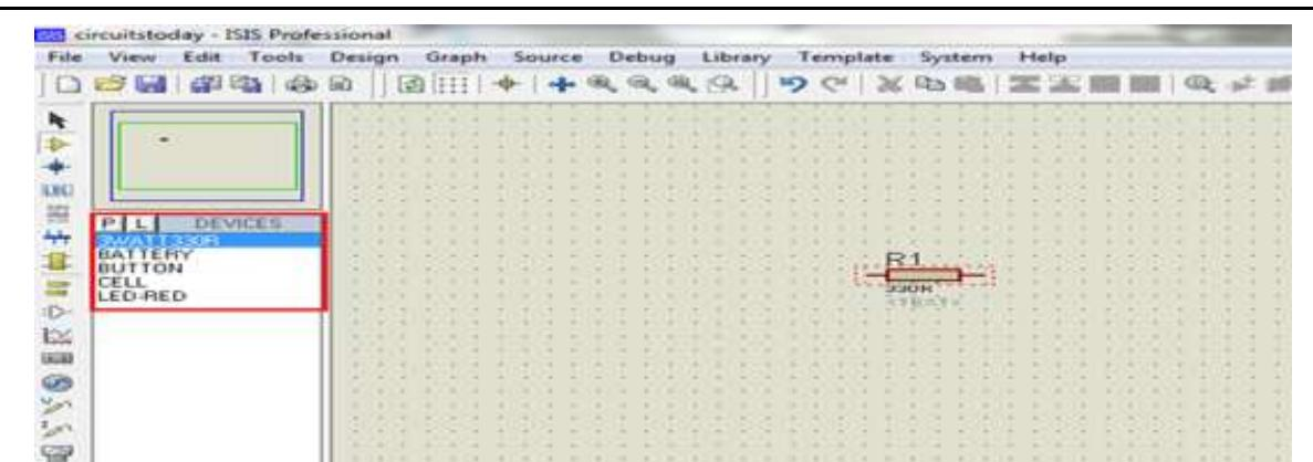
**Step5. Add Power Sources and Ground:** Go to the **Library** and search for **DC Voltage Source** or **Battery** and connect the ground to the relevant part of your circuit.
