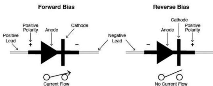
In the above diagram, we can see that there are two terminals that are known as anode
