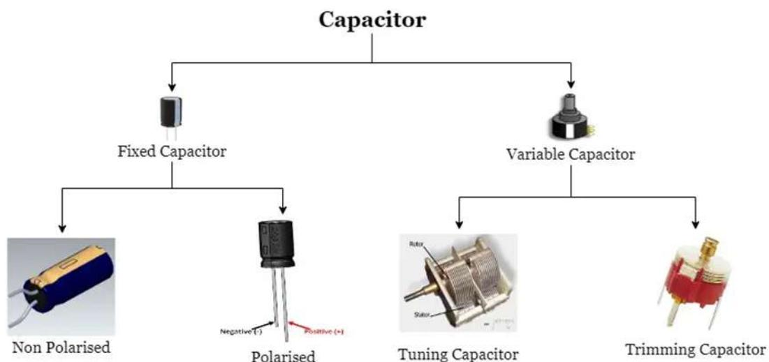
Many capacitors got their names from the dielectric used in them. But this is not true for all capacitors because some old electrolytic capacitors are named by its cathode construction.
