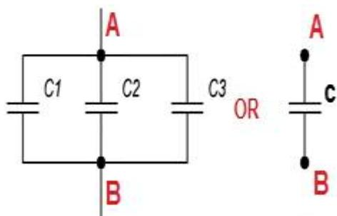
Since they are connected in parallel, they have the same voltage across their plates. But each capacitor can store different charges between their plates depending on their capacity. To find the equivalent capacitance of the combination, we first define the total charge  $Q$  stored by the combination. This is given as,
