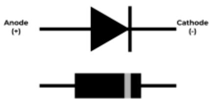
**Figure:** Symbol and overview of the Diode
