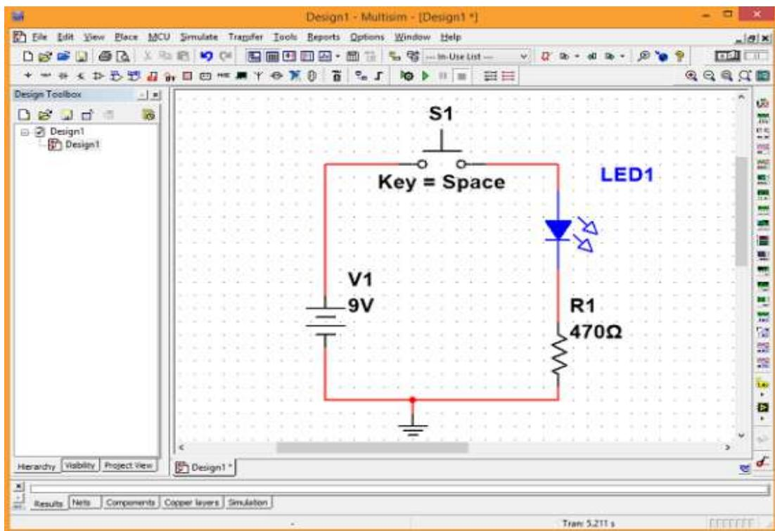
**Step 5: Add Ground and Power Sources:** Every circuit in Multisim needs a ground reference. Go to **Place > Component**, then search for "GROUND" under the **Sources** category and add a power source (e.g., DC voltage source) by selecting it from the **Sources > Power Sources** category.
