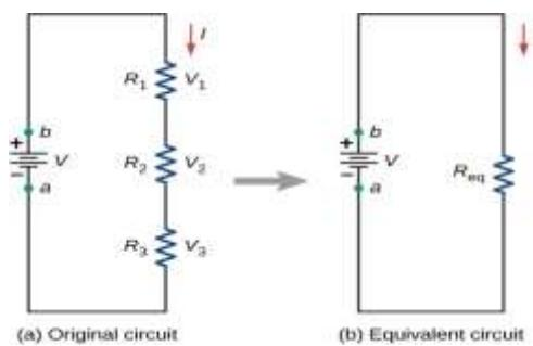
Figure (a) Three resistors connected in series to a Voltage source.
