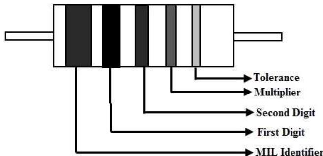
The table below shown gives the color corresponding to the numerical values for a five-band inductor.
