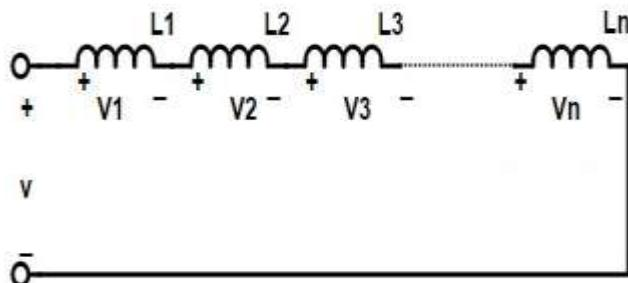
The inductance of series connected inductors is calculated as the sum of the individual inductances of each coil since the current change through each coil is same.
