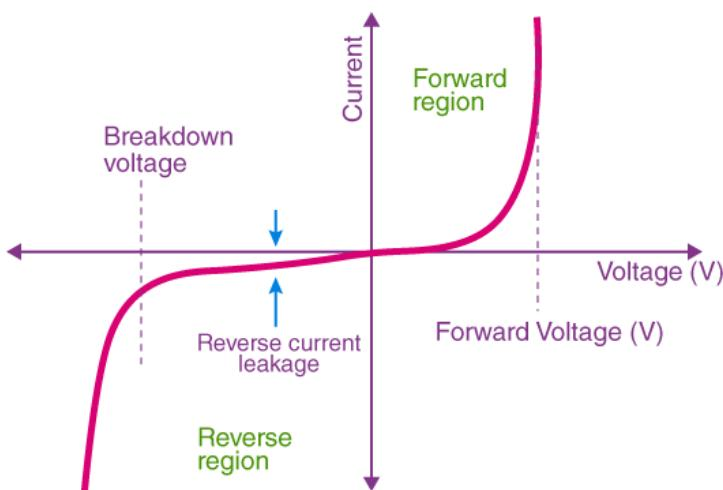
VI characteristics of P-N junction diodes are a curve between the voltage and current through the circuit. Voltage is taken along the x-axis while the current is taken along the y-axis.
