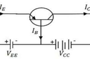
P-N-P Transistor biasing
