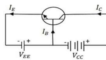
N-P-N Transistor biasing
