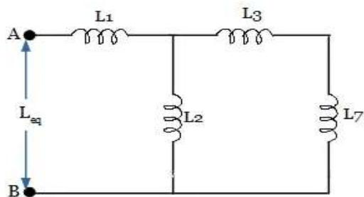
If you look at the circuit, inductor L2 is in parallel with the series combination of inductors L3 and L7. The corresponding equivalent inductance value is
