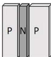
Construction of PNP & NPN Transistors
