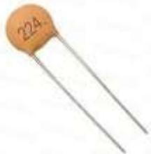
This capacitor has 224 written on it which gives the capacitance value of  $22 \times 10^4 = 220000$ pF or 220nF.
