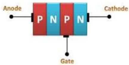
Thus, total four layers of semiconductor material are connected to each other and total three junctions are formed. In thyristors, there are three terminals that are anode, cathode and gate. Gate terminal provides the controlling voltage.
