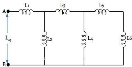
In the above example, inductor L4 is in parallel with a series combination of L5 and L6. The equivalent inductance value of these three inductors L4, L5 and L6 are
