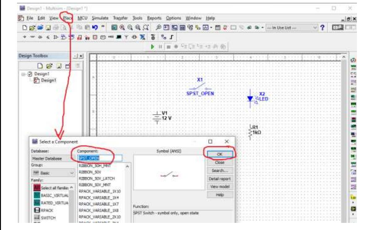
**Step 4: Wiring the Circuit:** Move the mouse pointer to a component's terminal (you'll see a crosshair), click and drag to another terminal to create a connection then after release the mouse button once the connection is established. Repeat for all connections.
