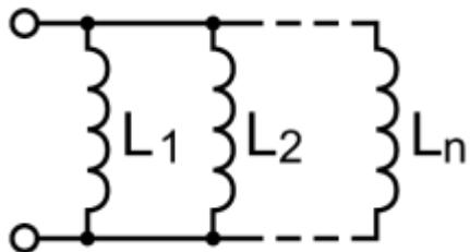
We know that, in a parallel network the voltage remains constant and the current divides at each parallel inductor. If  $I_{L1}, I_{L2}, I_{L3}$  and so on  $I_{Ln}$  are the individual currents flowing in the parallel connected inductors  $L_1, L_2$  and so on  $L_n$ , respectively, then the total current in the parallel inductors is given by
