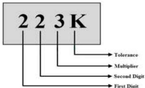
Suppose if an inductor is labeled as 223K, find the exact value of inductor.
