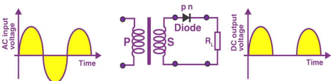
In the second half cycle, the current will flow from negative to positive and the diode will be reverse biased. Thus, at the output side, there will be no current generated, and we cannot get power at the load resistance. A small amount of reverse current will flow during reverse bias due to minority carriers.
