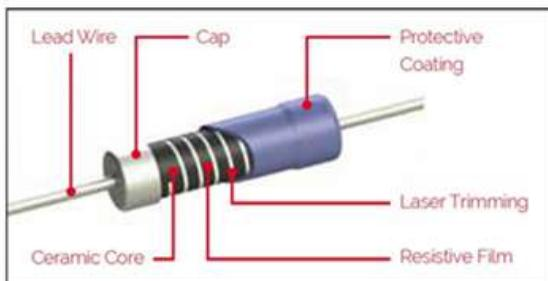
a) Construction of thin film resistor
