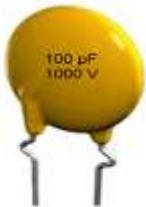
This capacitor uses ceramic as dielectric material (insulator). They are also known as multi-layer chip capacitor (MLCC) or disc capacitor. The values for ceramic disc capacitors vary from 1 nano farad to 1000 micro farad. They are mostly used in electronic circuits due to their low capacitance and resistance and better frequency response.
