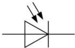
The symbol of the photodiode is similar to that of an LED, but here the arrow points inwards.
