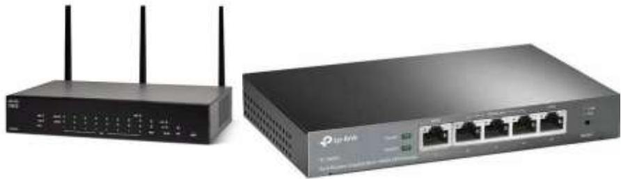
The router acts as a gatekeeper between the LAN and the Internet. It uses the Internet IP address itself and then provides computers on the LAN with their own IP addresses, which can't be seen outside of the LAN.
