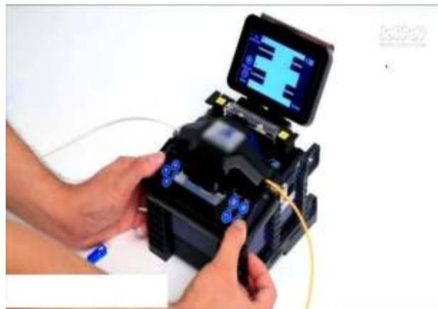
1. **Fusion splicing** machines join two pieces of material together by melting them together.
