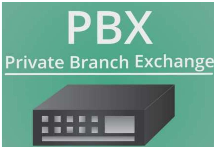
A PBX, or Private Branch Exchange, is a telephone system used by organizations to manage internal and external phone calls. It serves as a central switching system that connects multiple telephones within an organization, enabling internal communication and access to external phone lines, typically through a service provider. There are some key features and functions of a PBX system:
