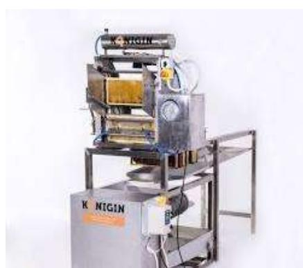
An uncapping machine is a device that uses a heated blade or roller to remove the wax cappings from honeycomb frames. This is a faster and more efficient way to uncap honeycomb frames than using an uncapping knife or a hot air blower.
