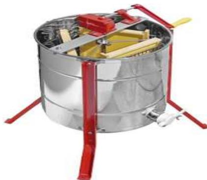
In tangential centrifugal extraction, the uncapped honeycomb frames are placed in the centrifuge basket with the sidebars facing outwards. The centrifuge is then spun at high speed, which forces the honey out of the honeycomb cells and into a container at the bottom of the centrifuge.
