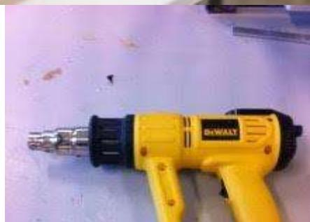
A hot air blower is a tool that produces a hot stream of air. It can be used to melt the wax cappings off of a honeycomb frame. This is a faster and easier way to uncaps honeycomb frames than using an uncapping knife, but it is important to be careful not to overheat the honey, as this can damage its flavour and quality.
