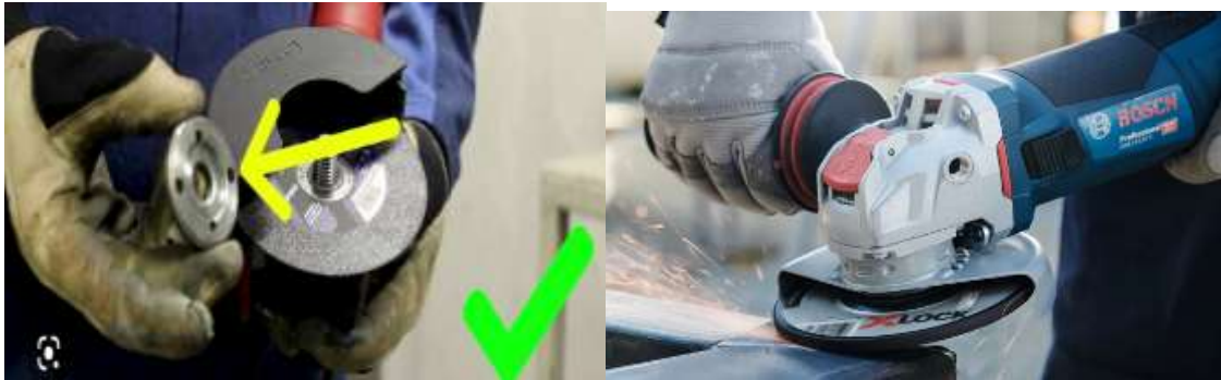
Figure 3: Inserting disc in angle grinder
