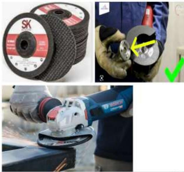
**Fig73:** Illustration of using angle grinder
