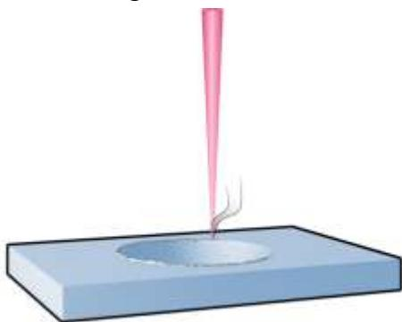
**Fig67:** Illustration of laser deburring
