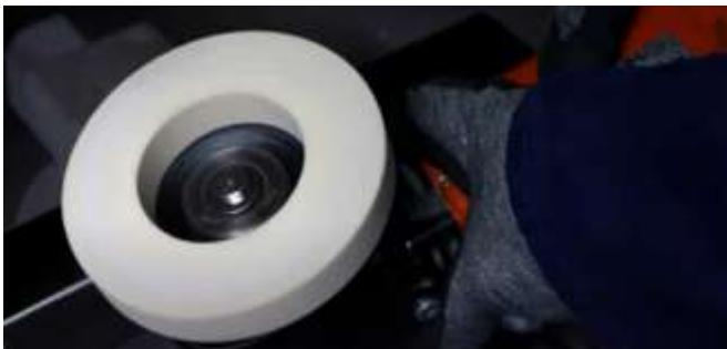
**Fig 75:** Polishing pad fitted into angle grinder
