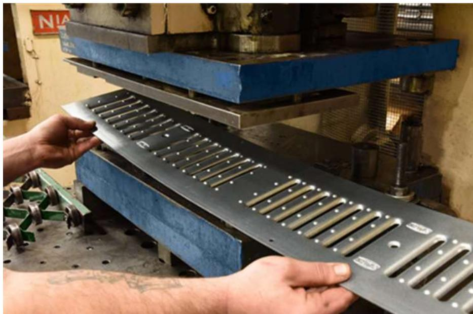
**Fig37:** Sheet Metal Stamping Process Aranda Tooling
