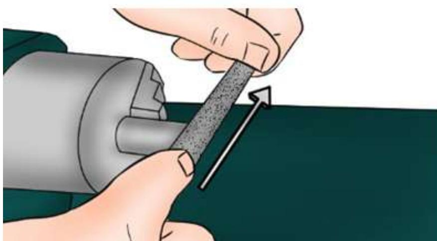
**Fig58:** Lathe deburring
