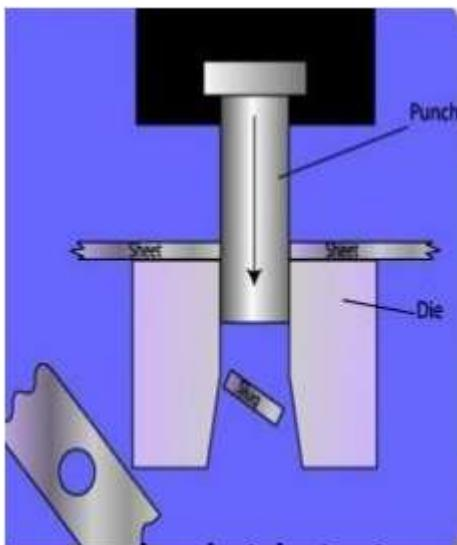
**Fig34:** Illustration of punching machine working principle.
