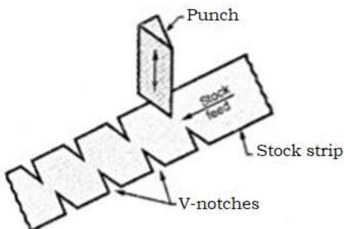
**Fig47:** Illustration notching operation
