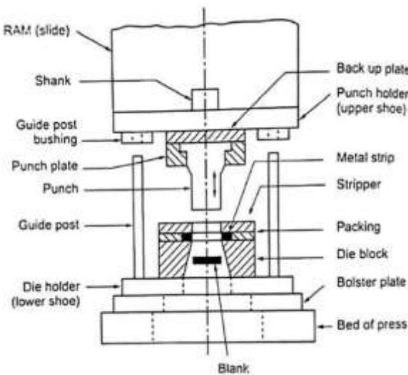
**Fig32: Hydraulic punching machine**
