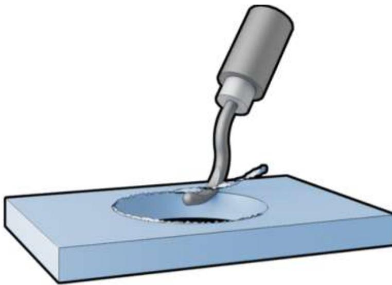
**Fig59: Illustration of Manual deburring**
