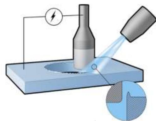
**Fig66:** Illustration of electro discharge deburring
