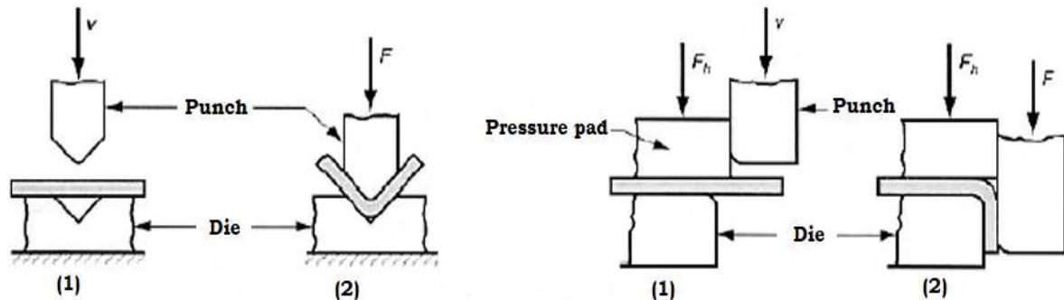
**(Left) V-bending, and (Right) edge bending ; (1) before and (2) after bending**
