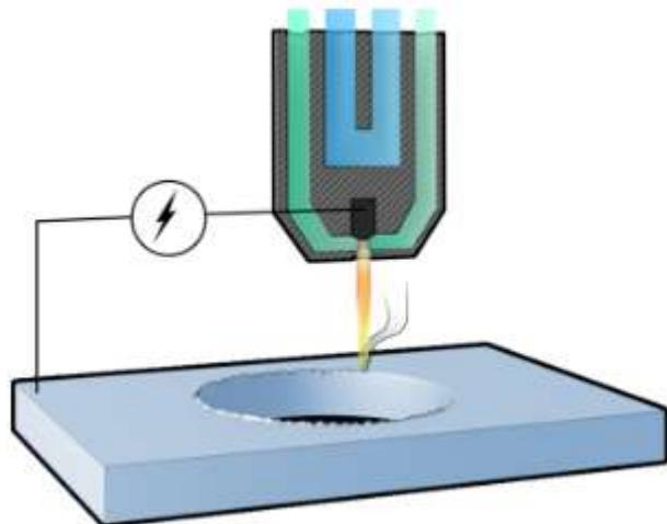
**Fig63:** Illustration of plasma deburring
