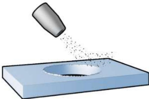
**Fig64:** Illustration of deburring with sandblasting
