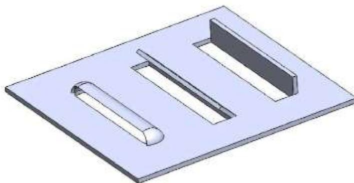
**Fig48:** Illustration of lancing operation
