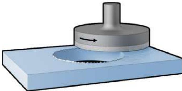
**Fig61:** Illustration of grind deburring
