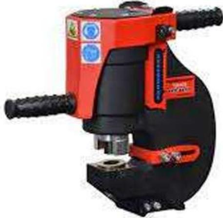
**Fig30:** Hand operated punching machine
