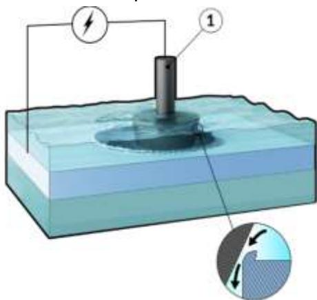
**Fig 65:** Illustration electrochemical deburring
