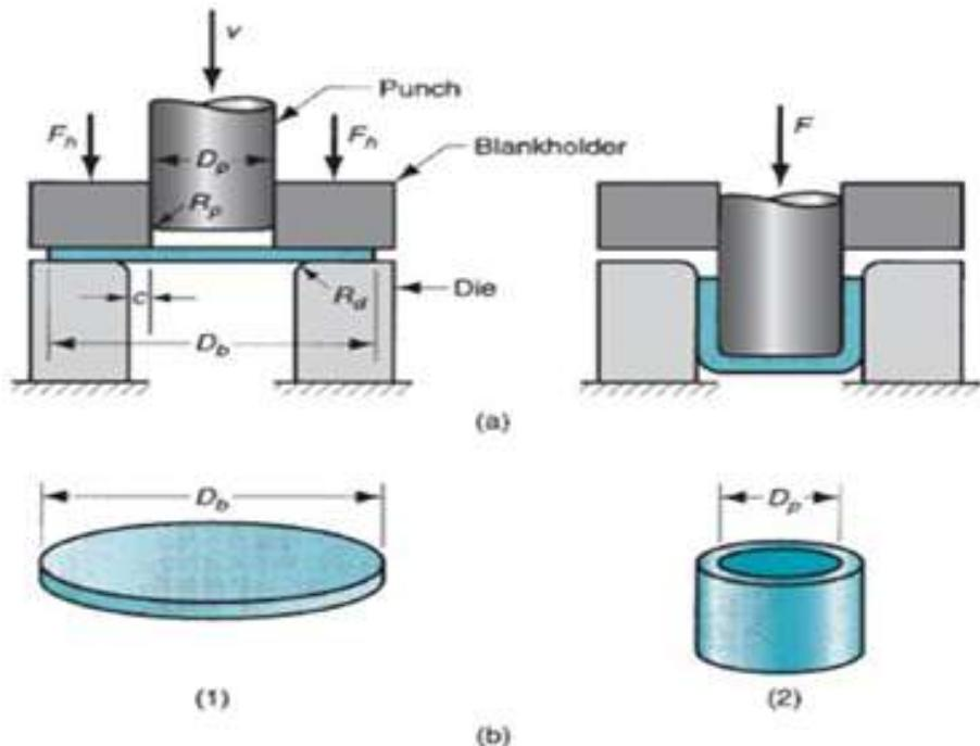
**Fig46:** Illustration of drawing operation
