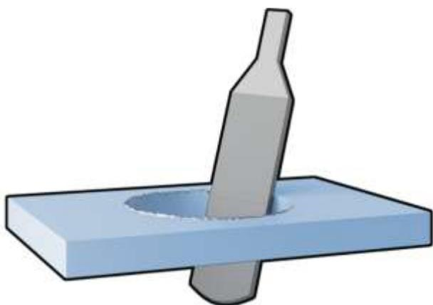
**Fig60:** Illustration of File deburring
