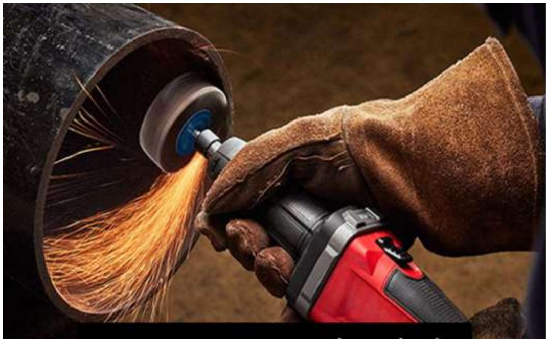
Die grinder is a simple yet powerful tool that is traditionally used to grind the metal. This tool is very versatile and can be used to grind almost any material. It is used to polish or smooth rough edges and has incredible power and unbelievable RPM speeds. It comes in both electric and pneumatic varieties. There are a number of jobs that a die grinder can help you with, but here are some of the most common uses.
