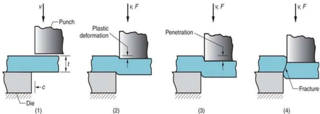
**Fig50:** illustration of punching phases
