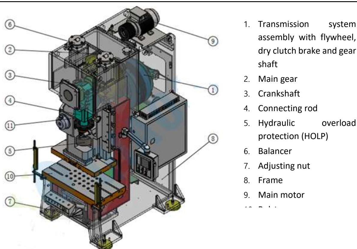
**Fig36:** Precision Single Crank C-Frame Stamping Machine.
