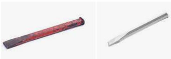
Wedge angle for soft materials 30 to 50 degree; for mild steel 60 to 70 degree; for alloyed steels 70 to 80 degree
