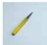
Punch marks are not only made to mark the scribed lines but also to determine insertion points for the dividers and hole centres.
