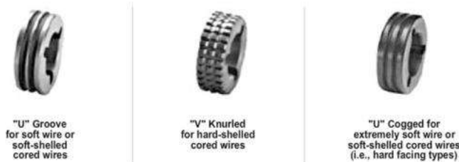
Figure 2.12. Drive roll types and applications.
