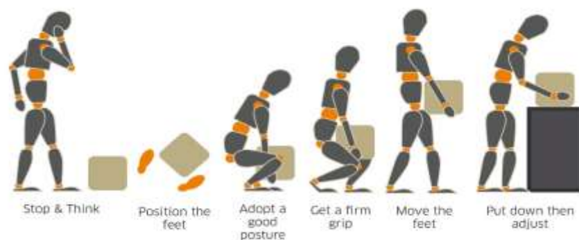
Figure 53: Procedures for safe manual handling
