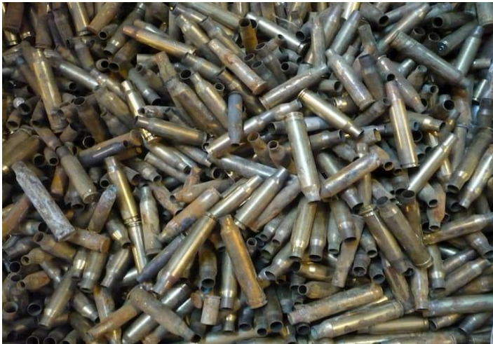
(Bullets container made in single phase brass)
