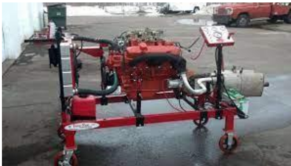
Figure 36: Testing the Engine for Run and Drive
