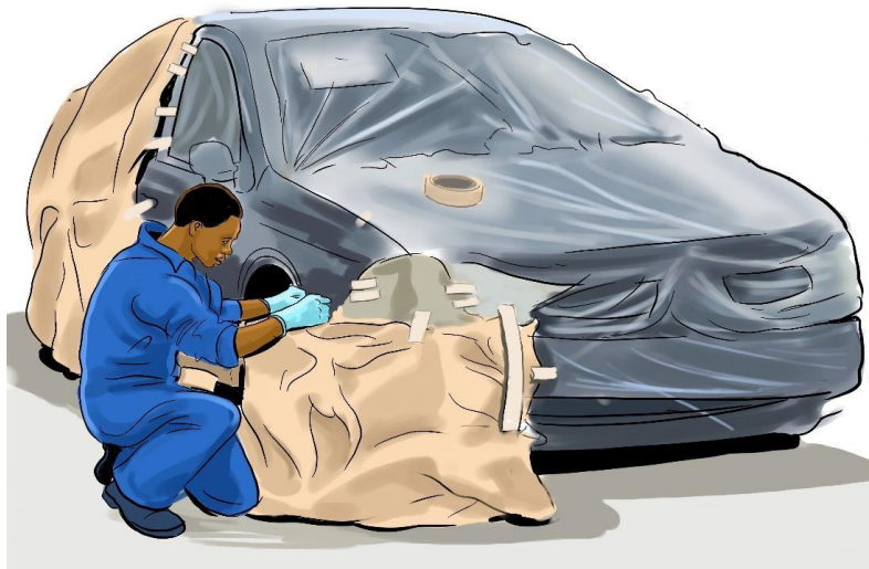
Figure 7: Technician is Covering unpaintable parts
