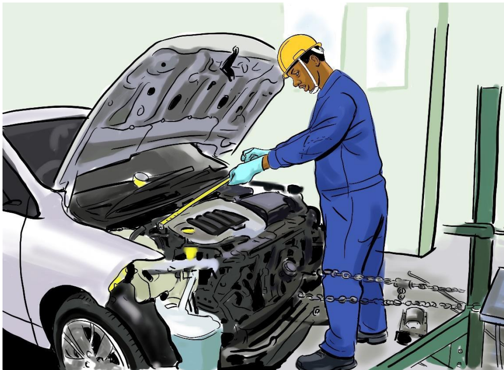
Figure 6: Technician is measuring the front damaged major part
