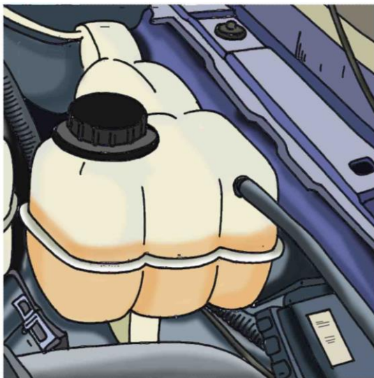
Figure 15: A coolant expansion tank
