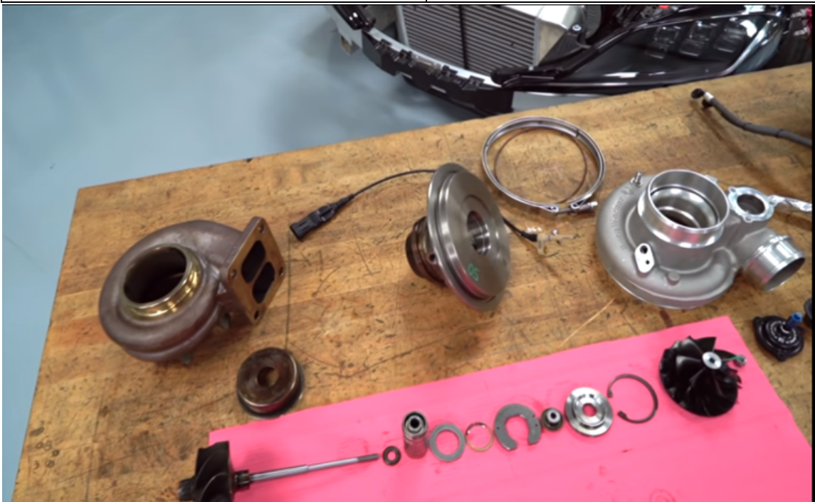
Figure 8: Steps to assembling and remount engine supercharging system
