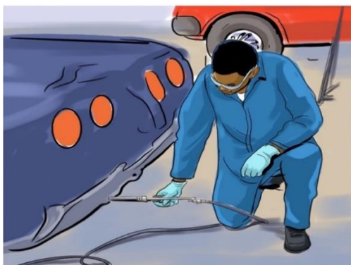
Figure 48 The analyzer's probe is inserted into the vehicle's tailpipe.
