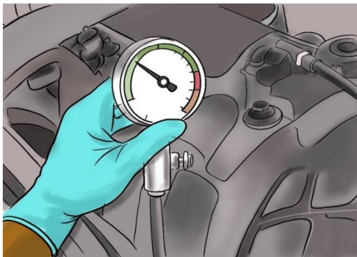
Figure 39 a vacuum gauge to test the exhaust system
