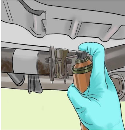
Figure 42 Spray the nuts along the exhaust pipe with penetrating fluid.
