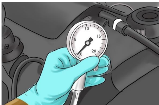
Figure 40 Backpressure gauge to test the exhaust system
