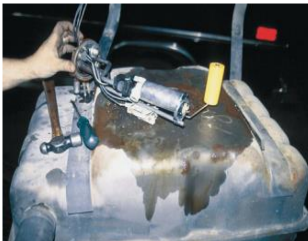
Figure 21: Fuel pump repair
