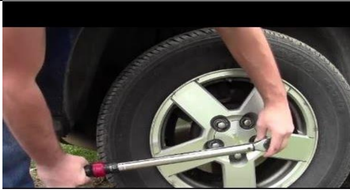
Figure 23: Wheel re-mounting with torque wrench
