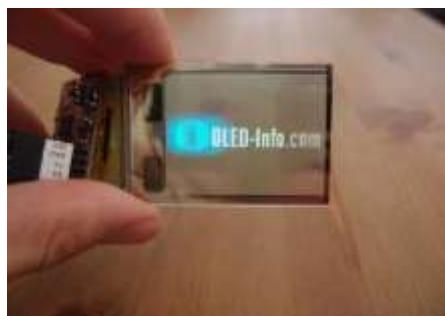
OLED is a technology that uses LEDs in which the light is produced by organic molecules. It is a flat light emitting technology, made by placing a series of organic thin films between two conductors. When electrical current is applied, a bright light is emitted.
