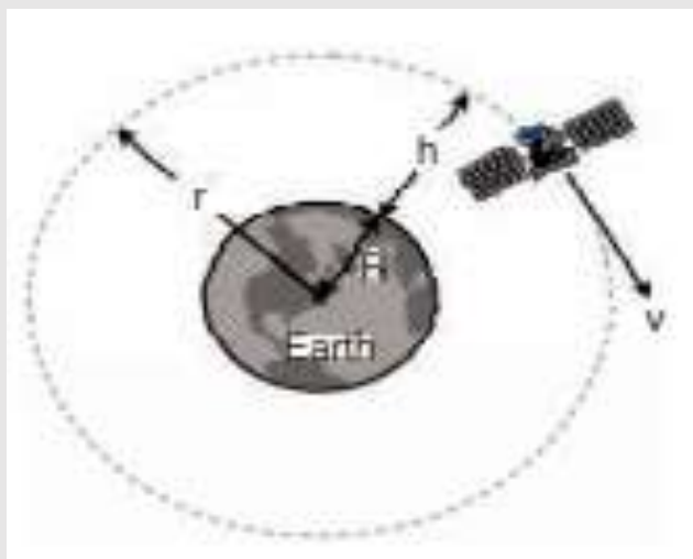
Figure 7: Orbital Velocity of Satellite.
