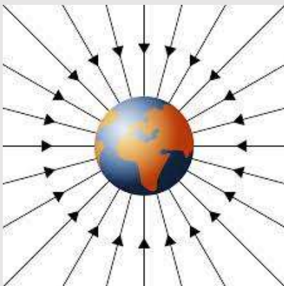
Figure : Gravitational field lines
