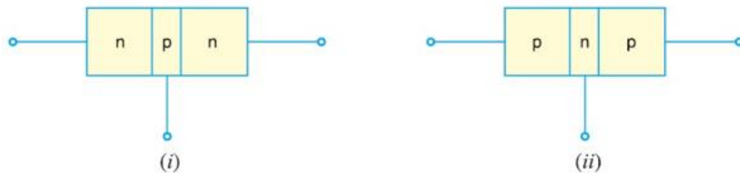
Figure 11: Structure of NPN and PNP
