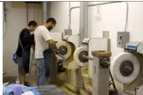
Buffers and buffing machines are **used to improve a surface's brightness or finish**. Buffers drive either non-woven abrasive pads or buffing pads that are loaded with buffing or polishing compounds. Centerless finishing polishers and buffing machines are used for grinding or finishing.
