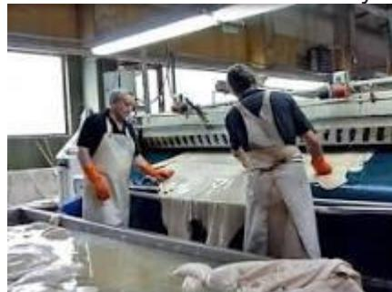
The drying of leather in the tannery. In the tannery, the leather is dried a maximum of two times between the many process stages. ...
