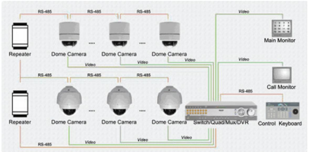
**NOTE:** To extend the network distance up to 1.2 km (4000 feet) and to protect the connected devices, it is highly recommended to place a repeater at the mid-point. However, a repeater may be needed in the network distance less than 1.2 km if the used cables are not the CAT 5, 24-gauge cables (see [3.4.4 RS-485 Connector](#)). Refer to the repeater's manual for detailed information.
