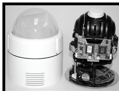
**Step 4:** Replace the dome housing with the cover back. Then screw it and the dome back together.
