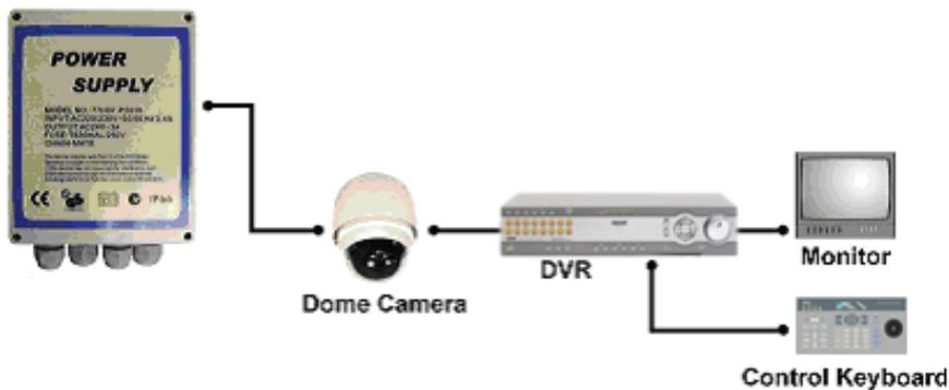
**NOTE:** One power box can only be connected to one outdoor dome camera subject to voltage restriction. In addition, up to two indoor dome cameras are allowed to be used with one power box.
