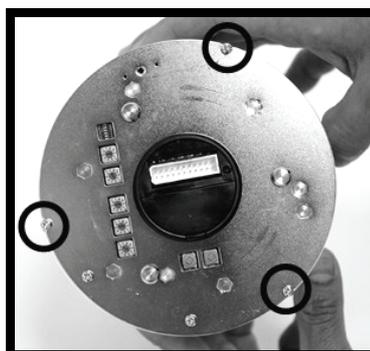
**Step 2:** Unscrew the three screws on the dome back, as marked in the figure, and remove the dome housing with the dome cover.
