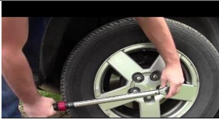
Figure 23: Wheel re-mounting with torque wrench
