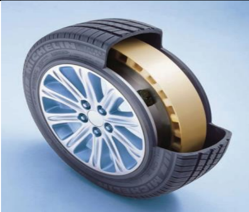
Figure 2: A cutaway of a run-flat tire with an insert to support the tire in case of air loss.
