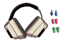
PPE includes ear muffs and plugs and should be used for tasks that can cause hearing problems and loss of hearing. Exposure to very loud noise levels for extended periods of time can lead to a loss of hearing. Air wrenches, engines running under a load, and vehicles running in enclosed areas can all generate annoying and harmful levels of noise.
