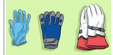
PPE includes safety gloves and should be used for tasks that can cause hand and skin burns, absorption of harmful substances, cuts, fractures or amputations.
