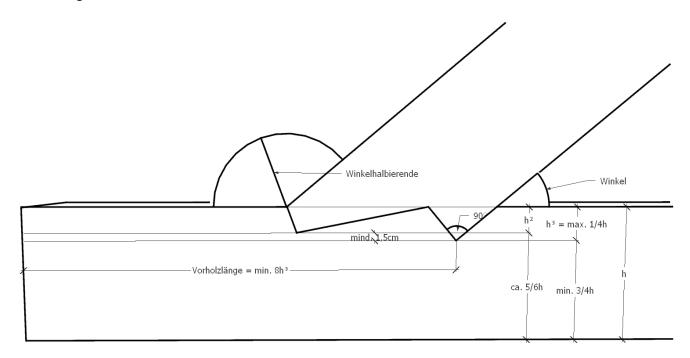
Even more stability is gained with this combination of the oblique thrust and the notched housing. It is important to keep in mind that the notched housing has to be at least one cm deeper than the oblique thrust. Otherwise both shearing planes would clash.
