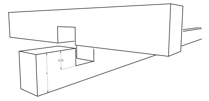
Any joint in which two pieces of wood are fixed across one another is called a cross joint. When cross-section weakening does not play a role both timbers can be notched up to half of their width.
