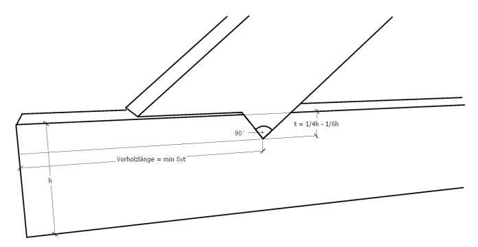
A notched housing should have a debth of 1/4 to 1/6 of the beam height. The beam projection requires a length of 8 times the debth of the notch or at least 20 cm.
