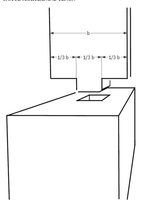
There are different sorts of tenons. A stub tenon is chiseled out over the whole width of the beam.
