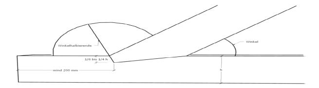
A wedge-shaped notch is cut into the load bearing beam. In this notch the compression beam is fitted.
