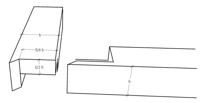
In some cases the end-grain should not be visible, either for weather related reasons or for the look itself. A concealed half-lap joint serves this purpose. It is manufacured similar to the half-lap joint, just adding some intermediate steps to hide the end-grain.
