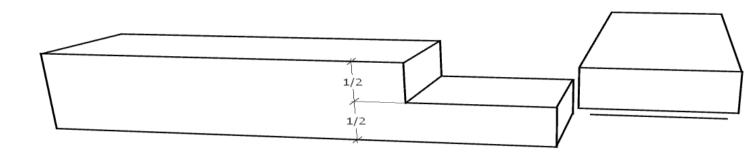
Similar to the halved scarf joint half of the beam width is cleared away. When joining the parts the surfaces are at one level.
