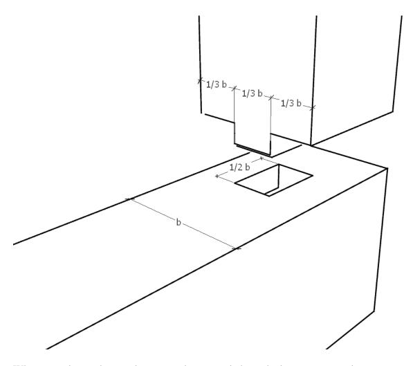
When some beams have to be mounted at an angle haunched tenons are used.
