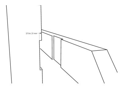
For creating a double notched joint both timbers are cut with notches to receive each other.
