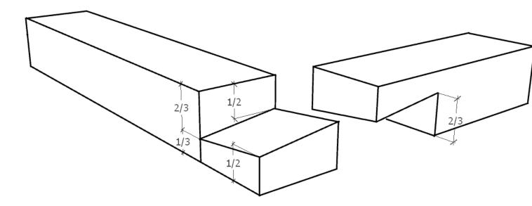
The bevel lap joint is one of the most complex corner joints. Because it has an oblique surface it is not as easy to draft as the half-lap joint.
