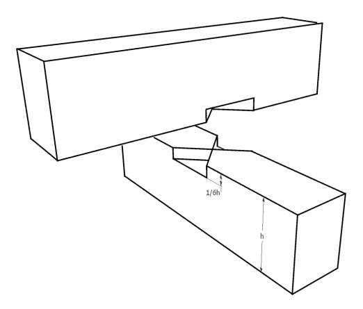
Drafting this joint is easy: By joining the particular timbers and the connecting of the four corners a cross is formed.
