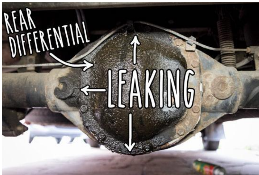
Figure 165: Check the rear differential for leakage
