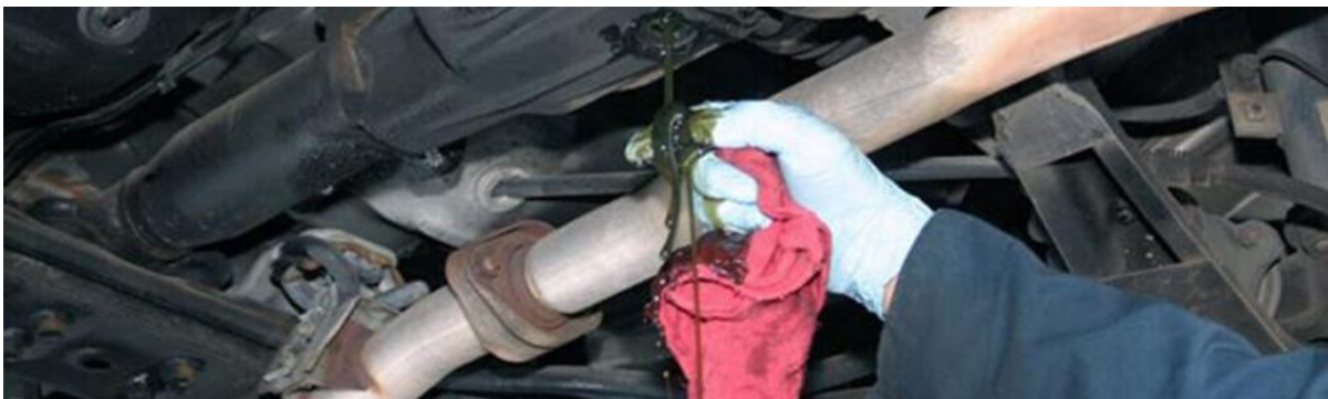
Figure 159: Locate the differential drain bolt. Loosen and remove
