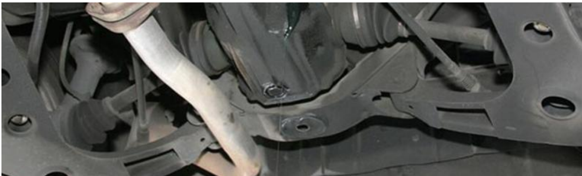
Figure 162: Add a recommended gear oil.
