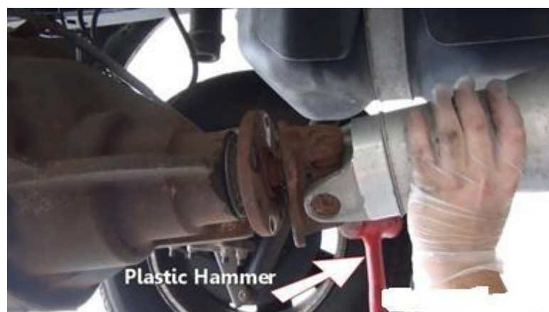
Figure 12: Use a plastic hammer to remove driveshaft flange
