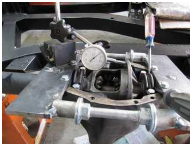
Figure 129: Carrier bearing measurements
