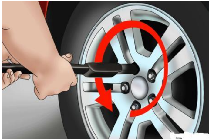
Figure 20: Loosen the lug nuts of the wheel
