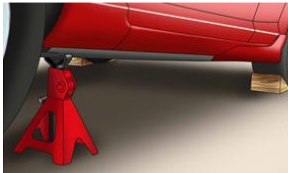
Figure 21: Jack stand to support the vehicle
