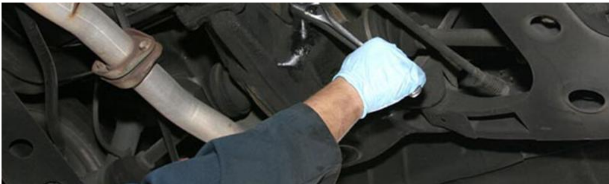
Figure 163: Reinstall and tighten the fill hole bolt
