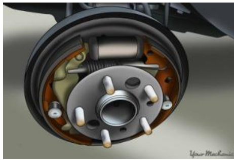
Figure 32: Reinstallation the tensioning springs
