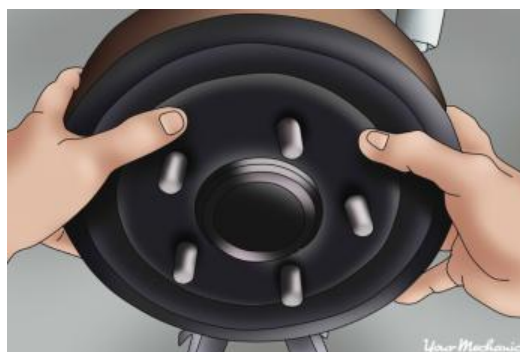
Figure 36: Installation of the drum brake over the brake shoes
