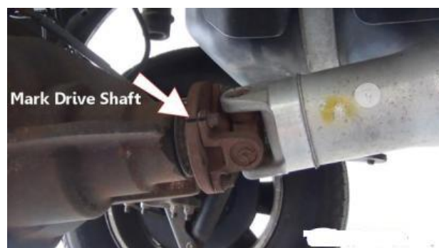
Figure 10: How to mark a drive shaft
