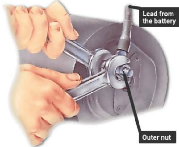
Figure 42: Hold the terminal-post but with a spanner while you unscrew the outer nut securing the lead from the battery.
