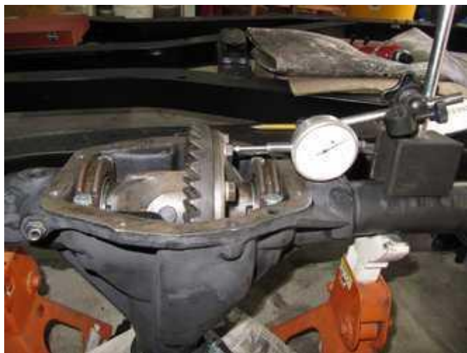
Figure 135: Measuring carrier bearing
