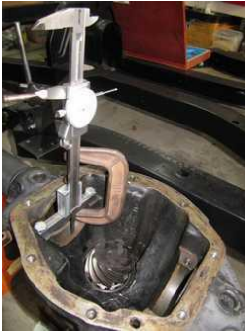
Figure 127: measuring clamp with Vanier caliper
