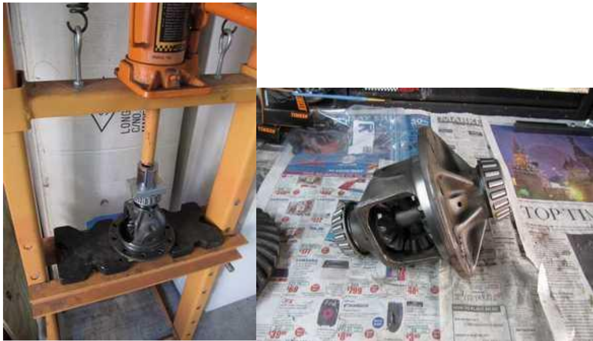
Figure 128: Use press to install carrier float
