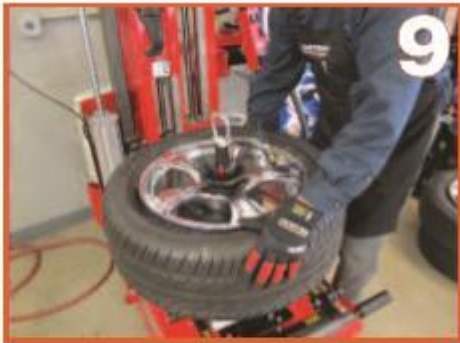
Seat both beads using air pressure and a gentle lift of the tire up into the top rim flange.
