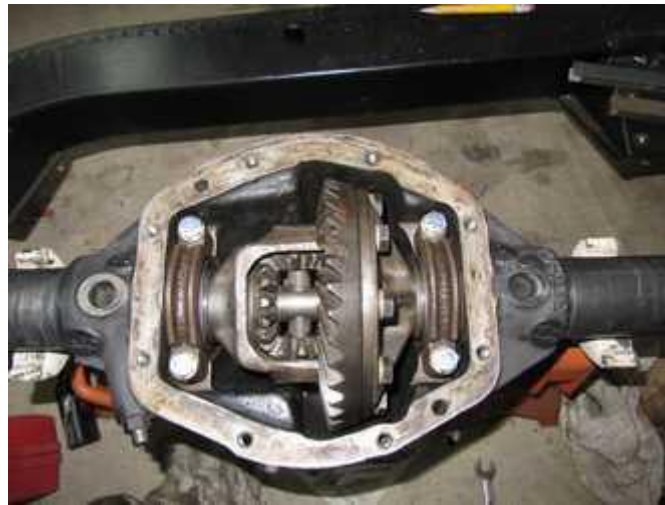
Figure 138: A hauled out my case spreader, spread the case, and dropped the carrier into position. I installed new bolts for the bearing caps. Finally, I rechecked the backlash and measured 5 mils. Done! Below is the finished differential.
