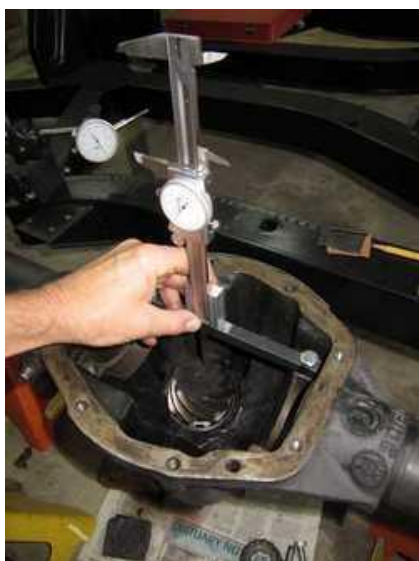
Figure 134: To determine the distance from the carrier center to the bearing-contact surface of the pinion gear.
