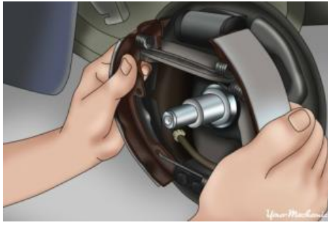
Figure 31: To secure the new brake shoes onto the hub
