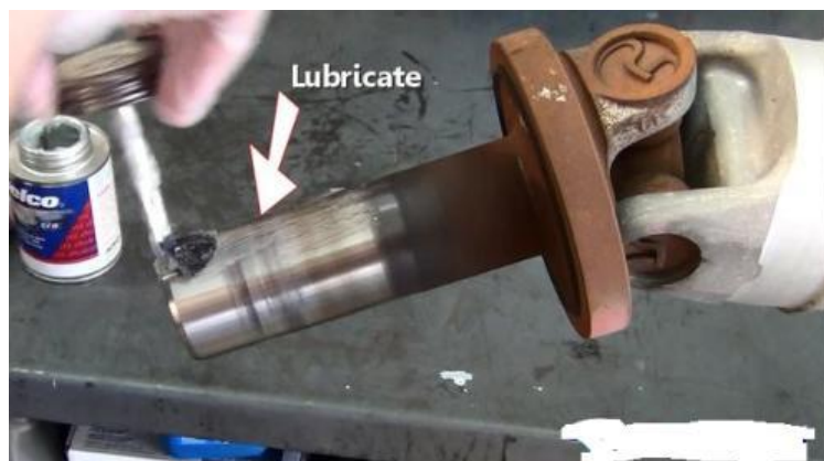
Figure 14: lubricate a driveshaft
