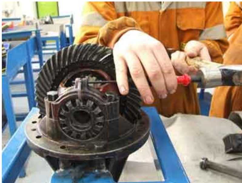
Figure 140: Use the correct tool provided in order to preload the Crown wheel carrier bearings. These bearings must be preloaded, but the position of these bearings also controls the position of the Crown wheel, and thus the Crown wheel to pinion backlash. When the bearings are correctly set, knock out the roll pin from the locking lever.
