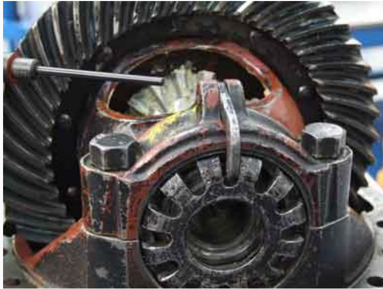
Figure 73: use proper tool to remove roll pin lever
