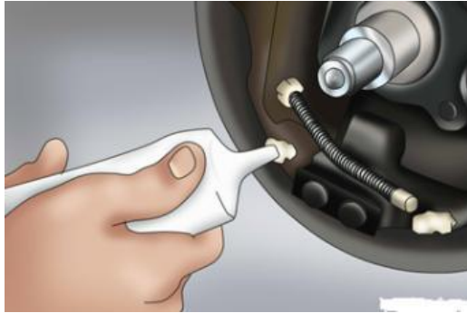
Figure 28: Clean the backing plate with brake cleaner
