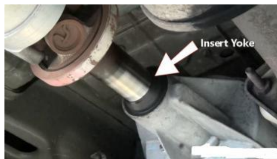
Figure 16: Insertion of Yoke in driveshaft
