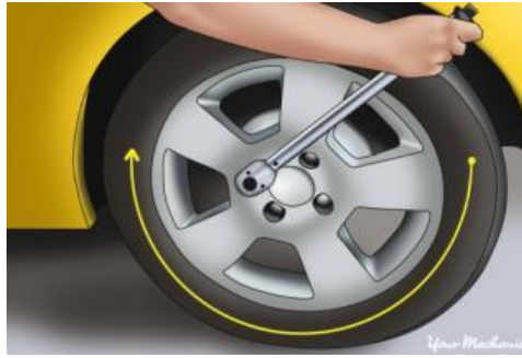
Figure 39: Torque the wheel lug nuts to specification
