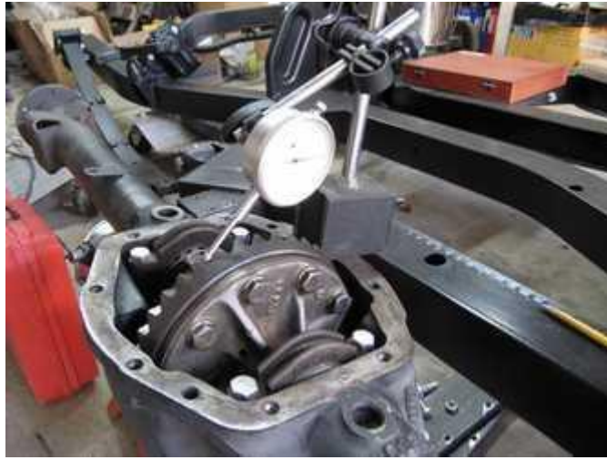
Figure 136: The total float measurement
