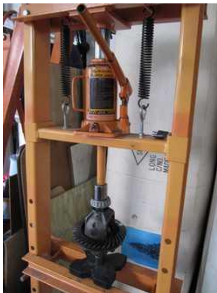
Figure 137: Use press to insert the carrier.
