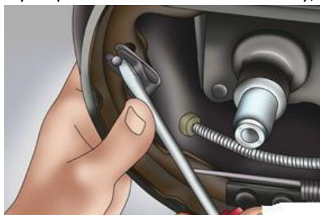
Figure27: The parking brake cable retainer clip removal
