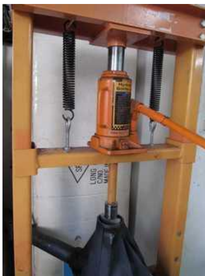
Figure 131: use press to set up shims and outer bearing cone
