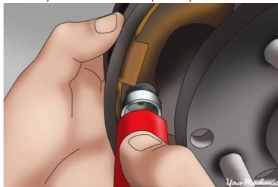
Figure 33: Installation of the hold down pins and springs.
