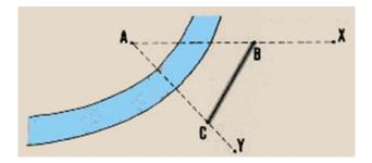
Figure: Measuring horizontal angle when you cannot reach the summit of the angle A
