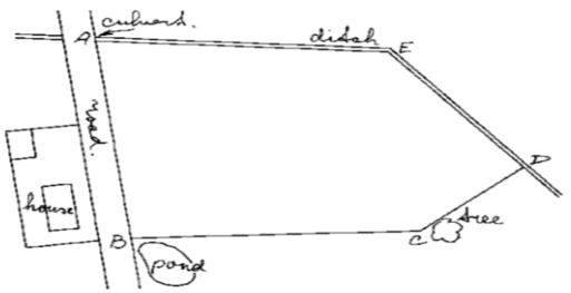
Figure: A field with an irregular shape of which the surface area must be determined.
