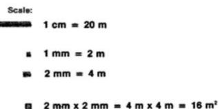
Figure: Area calculation using square-grid method
