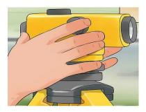
Figure: Check level's calibration by turning it 180 degrees
