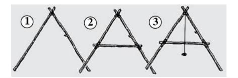
Figure: These pictures show how the A-Frame is put together.
