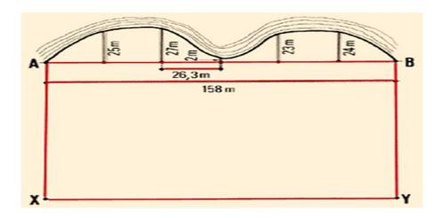
Figure: example of area culcuration for area bounded by curve
