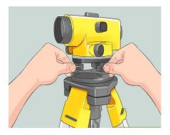
Figure: Levelling the device by adjusting the 2 leveling screws
