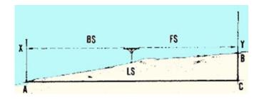
Figure: Difference in elevation from BS-FS
