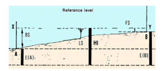
Figure: Elevation of unknown point by HI-FS
