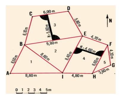
Figure: area calculation without common base
