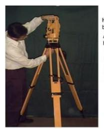
Hold Theodolite by handle Attach to tripod head Do not let go of handle until theodolite is attached to tripod.
