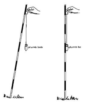
Figure: Wrong and Right placing a ranging pole
