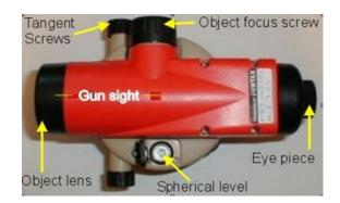
Figure: Main parts of a dumpy level (right side) Figure: Main parts of a dumpy level (top view)
