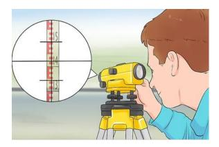
Figure: Adjusting of eyepiece to see the device's crosshairs
