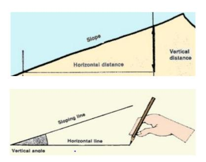
Figure: Vertical angle; vertical distance; horizontal distance and land slope
