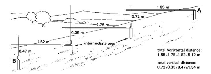
Fig: Measurement of horizontal and vertical distances when using intermediate pegs, Step 2
