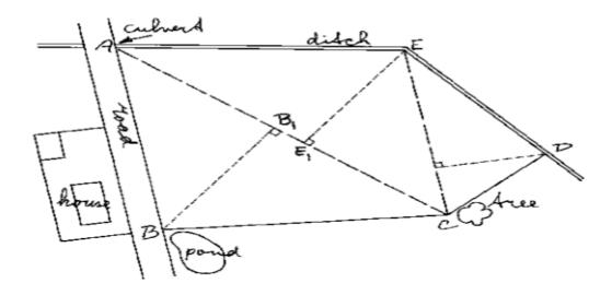
Figure: Irregular field divided into regular shapes
