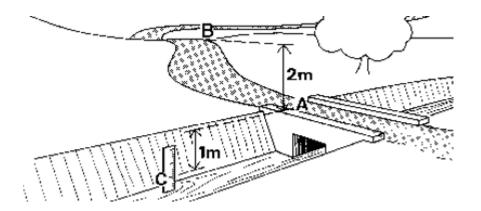
Figure: Vertical distance or height difference from reference point or datum "A"
