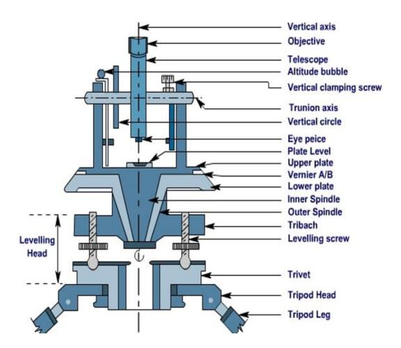
Figure: Main parts of a Theodolite
