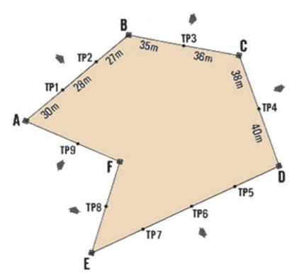
Figure: Closed differential survey
