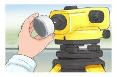
Figure: Removal dumpy level's lens cap
