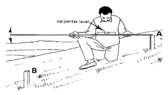
Fig: Measurement of horizontal and vertical distances, Step 2
