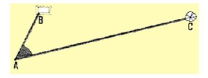
Figure: Horizontal angle BAC
