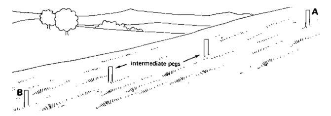
Fig: Measurement of horizontal and vertical distances when using intermediate pegs, Step 1
