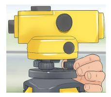
Figure: Adjusting the third leveling screw
