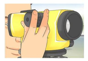
Figure: Twisting the device's focusing knob until the image is clear
