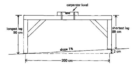
Figure: N frame level adjustment by reducing the leg height for measuring slope
