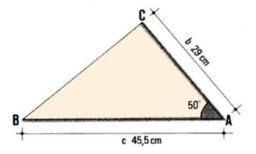
Figure: Area calculation using Sin method
