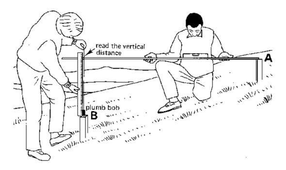
Fig: Measurement of horizontal and vertical distances, Step 4
