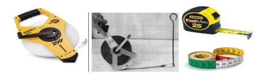
Figure: Different forms of tape measures
