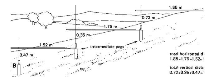
Fig: Measurement of horizontal and vertical distances when using intermediate pegs, Step 2
