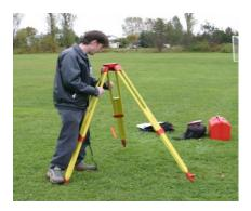
Figure: Checking that the tripod head is approximately level and the tripod feet are firmly fixed in the ground.
