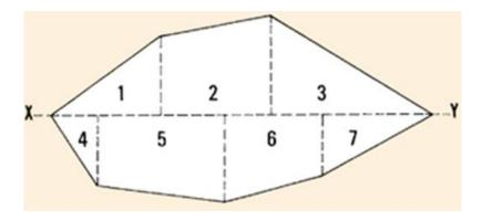
Figure: A base line X,Y used to subdivide land area
