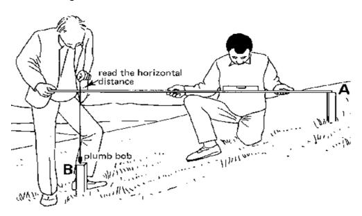
Fig: Measurement of horizontal and vertical distances, Step 3
