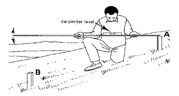
Fig: Measurement of horizontal and vertical distances, Step 2
