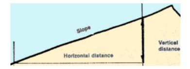
Figure: Land slope; horizontal distance and vertical distance
