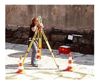
Figure: Theodolite in use with cones to protect tripod positioning
