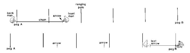
Figure: Arrows used in long distance measurement
