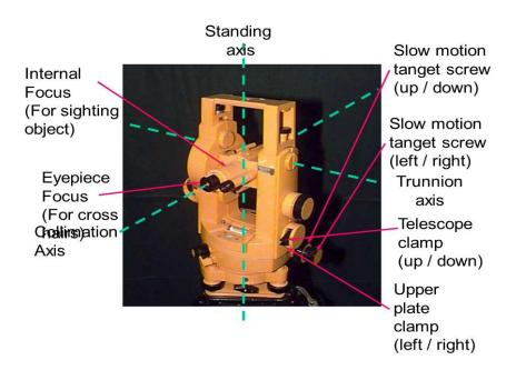
Figure: Different theodolite axis
