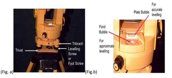
Figure: Theodolite levelling main parts
