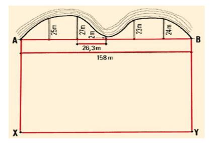
Figure: example of area culcuration for area bounded by curve
