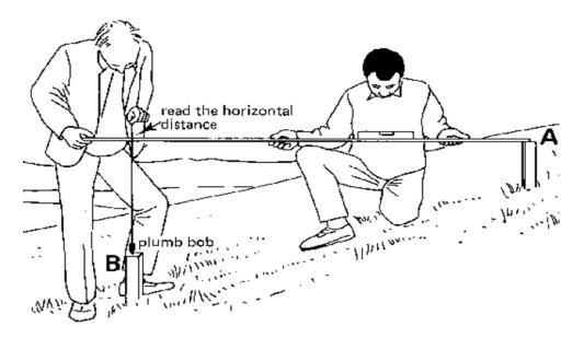
Fig: Measurement of horizontal and vertical distances, Step 3
