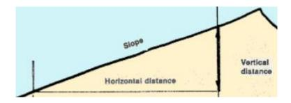
Figure: Vertical distance; horizontal distance and slope
