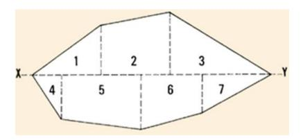
Figure: A base line X,Y used to subdivide land area
