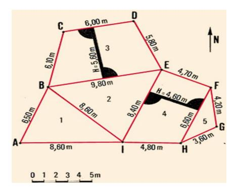
Figure: area calculation without common base
