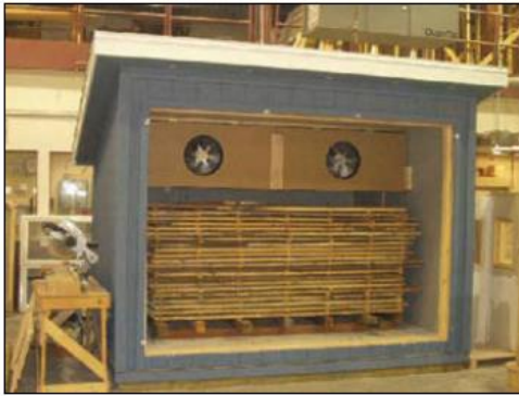
Figure 6—Dehumidification dry kiln loaded with air-dried mixed hardwood and softwood.
