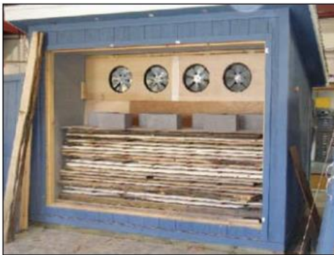
Figure 7—Dehumidification dry kiln loaded with green mixed hardwood (four fans are shown, because two were added).
