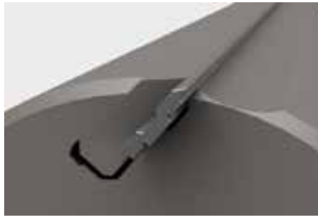
Fixed by form: groove (TERSA)
