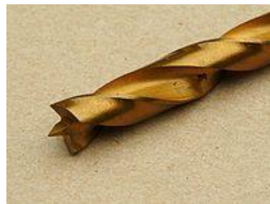
Point angel bit for exact centering only used for wood
