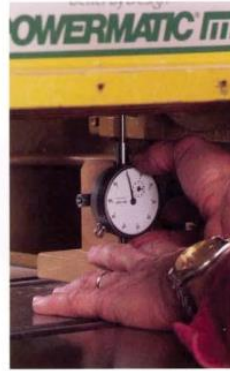
Move the indicator to one side of the cutterhead and adjust it so it reads zero.
