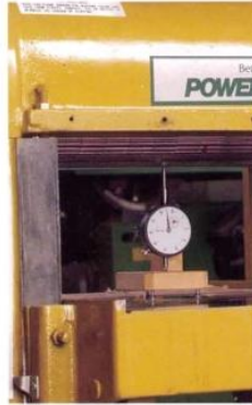
To check cutterhead alignment, start by adjusting the table to bring the indicator's hand to the vertical position after it has made a couple of turns.
