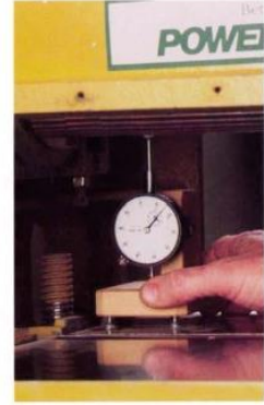
Move the indicator to the opposite end of the cutterhead and take another reading. Here the head is out of parallel by 0.005 in.
