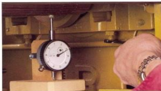
Set infeed and outfeed roller height by adjusting screws at each end of the rollers after taking a measurement with a dial indicator.
