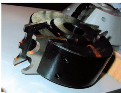
Figures 1a & 1b Round form tool with limited cutter projection
