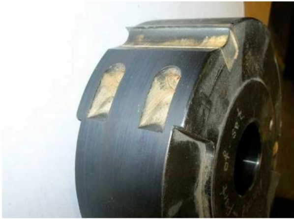
Figure 7 Key or wedge-shaped cutter
