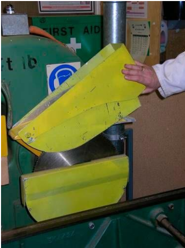
Figure 2 Additional gravity fall guard, made by the duty holder, fitted to the cut-off saw of an older machine
