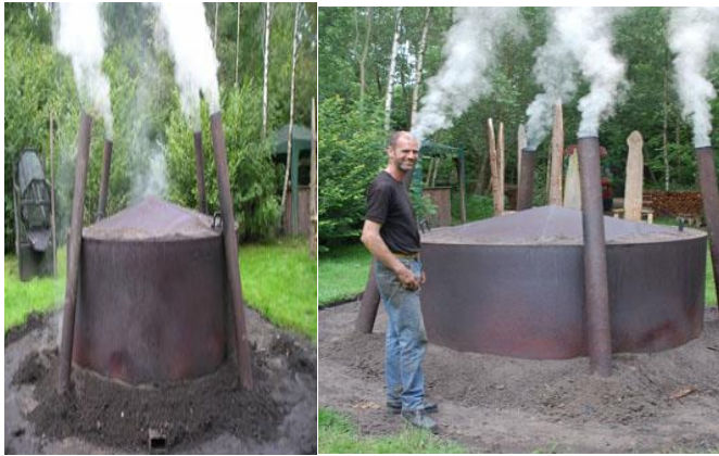
Figure 10: Carbonization process of metal kiln
