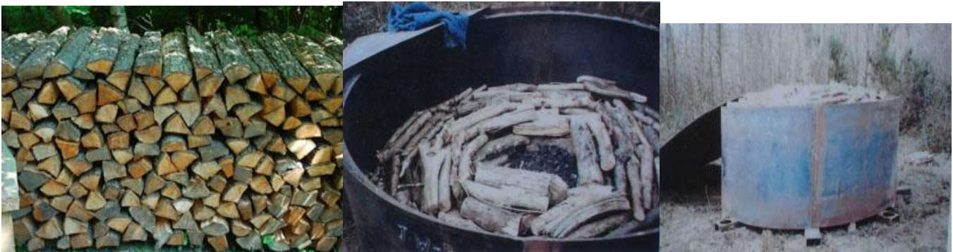
Figure 8: Metal kiln loading system
