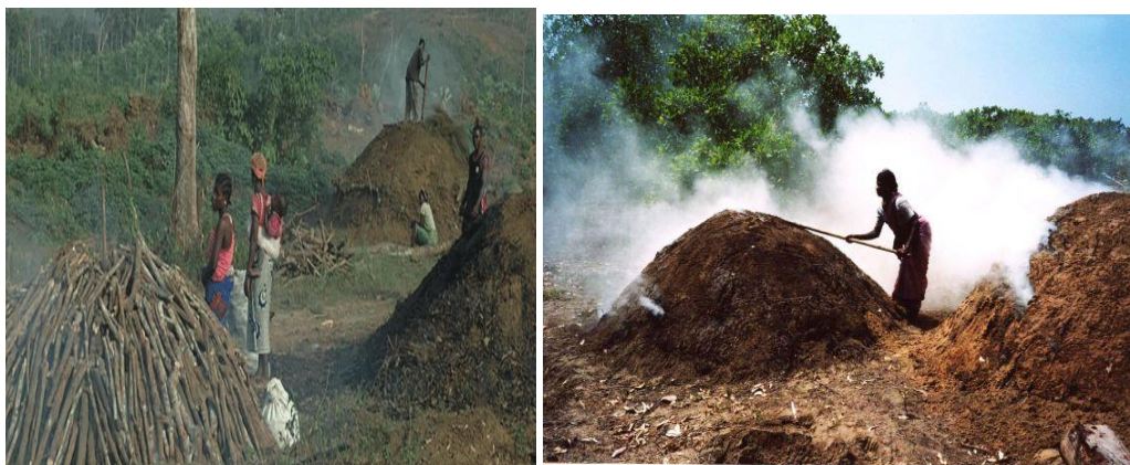
Figure 2: Construction of Earth mound kiln
