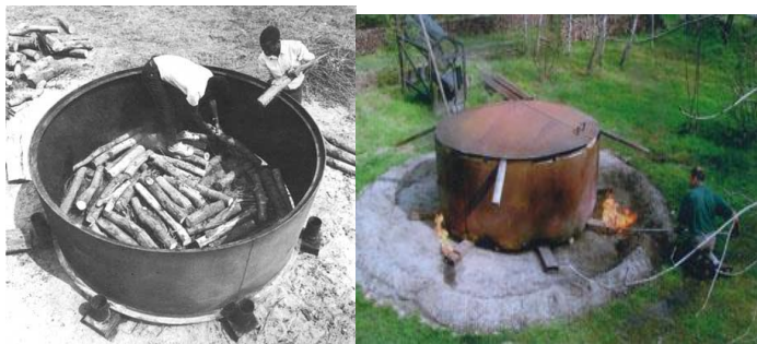
Figure 4: Wood charging operation on left side and a well ignited metal kiln on right side
