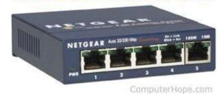
Like Hub, switch don't broadcast the received message to entire network, rather before sending it checks to which system or port should the message be sent. In other words switch connects the source and destination directly which increases the speed of the network.
