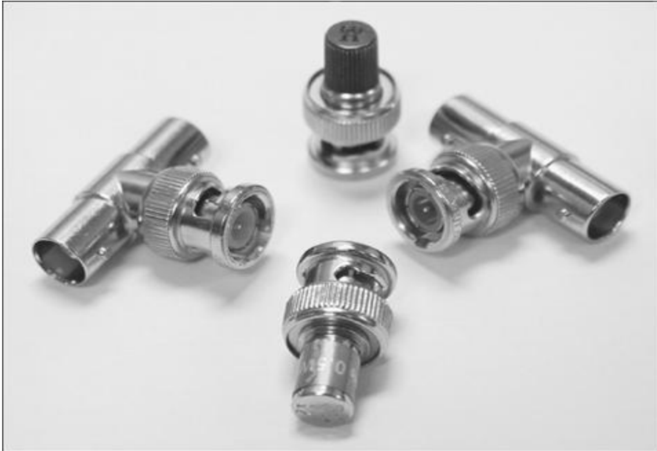
Fig.16: Two terminators (top and bottom) and two T-connectors (left and right)
