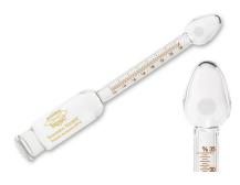
2. Fill the 10.75 ml pipette with milk and deliver the sample into butyrometer.
