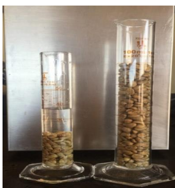
Fig7: Graduated cylinder for measuring density
